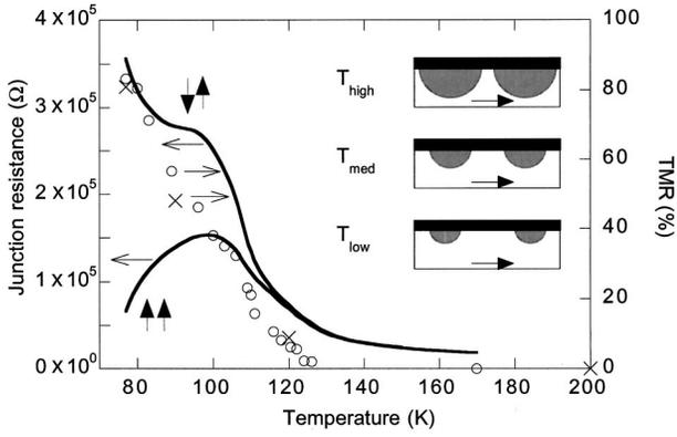
FIG. 4. The temperature dependence of the junction resistance in parallel (1000 Oe) and antiparallel (350 Oe) spin configurations (continuous lines) and the corresponding temperature dependent tunnel magnetoresistance for two different junctions (symbols). The inset schematically illustrates the growth, with decreasing temperature, of interconnected ferromagnetic regions (unshaded) next to the tunnel barrier (black).
