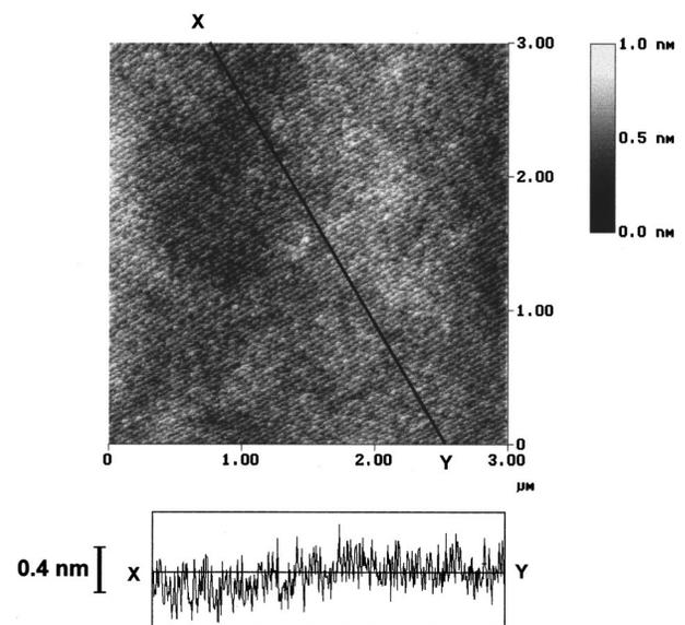
FIG. 1. The surface AFM image of the LCMO/ $\text{NdGaO}_3$ /LCMO trilayer ( $3 \times 3 \mu\text{m}^2$ ). The cross-sectional line profile shows that each step height corresponds to one unit-cell thickness of pseudocubic perovskites in a given heterostructure.
