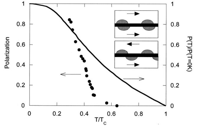
FIG. 5. The temperature-dependent polarization derived from the observed TMR using Eq. (2) is compared to the spin anisotropy of a  $\text{La}_{0.7}\text{Sr}_{0.3}\text{MnO}_3$  thin film measured by spin-polarized photoemission (reproduced from Ref. 16). The inset shows a schematic diagram of the tunnel device with phase separated paramagnetic regions adjacent to the barrier shaded gray. The ferromagnetic regions (unshaded) merge further into the electrodes as the effective local  $T_C$  rises.
