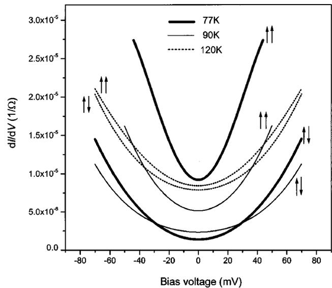
FIG. 3. The dynamic conductance  $dI/dV$  of junction (1) from Fig. 1(b) versus bias voltage for parallel (1000 Oe) and antiparallel (350 Oe) spin states at different temperatures. All curves can be accurately fitted by a function of the form  $dI/dV = A + BV^2$ , where  $A$  and  $B$  are constants which depend on the temperature and magnetization alignment.
