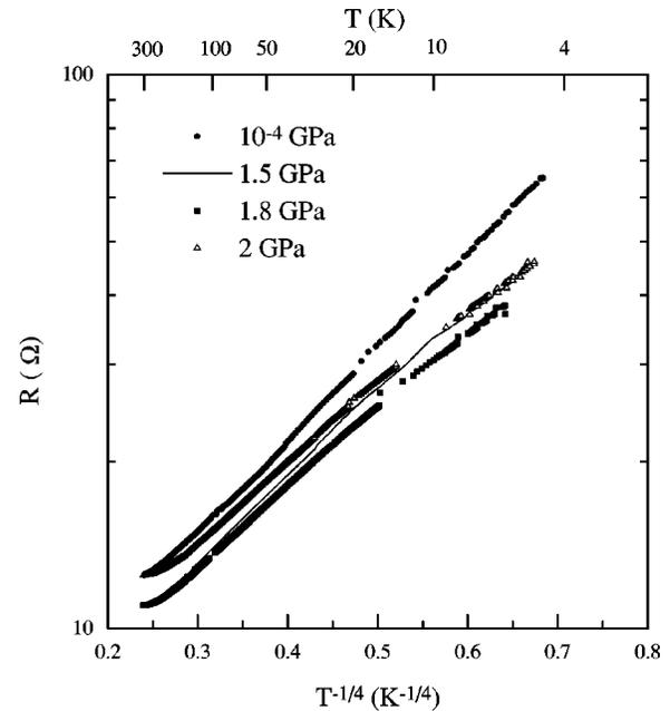
FIG. 4. Temperature dependence of the resistivity measured at different hydrostatic pressures. Plots show  $\log(R)$  as a function of  $T^{-1/4}$  in order to demonstrate hoppinglike conduction.
