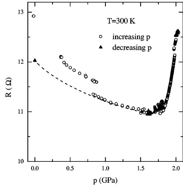
FIG. 2. Pressure dependence of the room temperature resistivity. Circles are points taken upon increasing pressure, triangles upon decreasing. Upon increasing the pressure we have made  $R(T)$  measurements at 0.8, 1.5, 1.8, and 2 GPa. The discontinuity in the curve at 0.8 GPa is due to this interruption and we think that it reflects the annealing of the sample.
