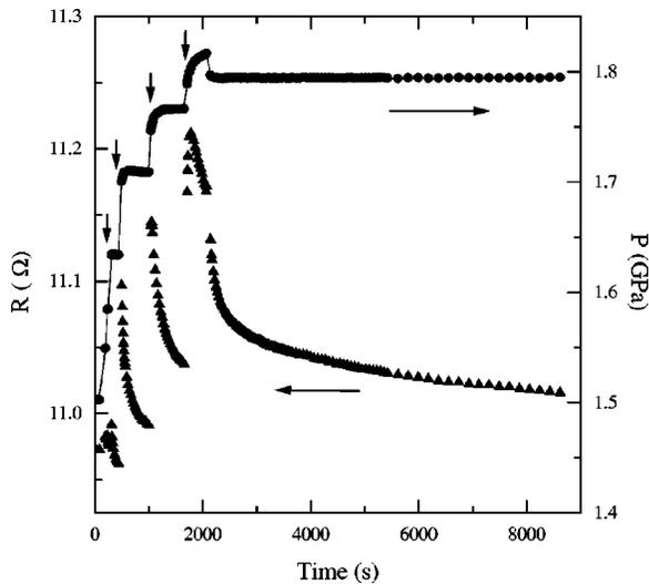
FIG. 3. Relaxation of resistance in the 1.5–1.8 GPa pressure range. The right-hand scale shows the pressure, the left-hand scale the sample resistance as a function of time. Arrows indicate where pressure was raised.
