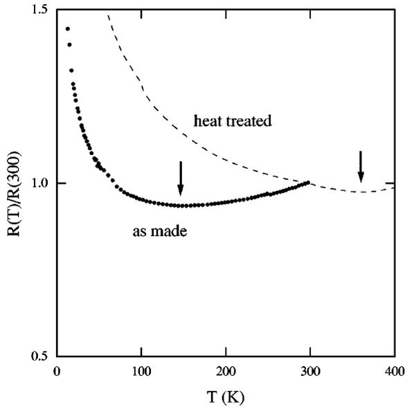
FIG. 1. Temperature dependence of the resistivity of a chemically purified and filtered buckypaper and one that received an additional heat treatment in vacuum at 1200 °C. One can note the shift of the minimum of the resistivity,  $T^*$  to higher temperature. Upon the heat treatment sample resistivity has increased by a factor of 5.
