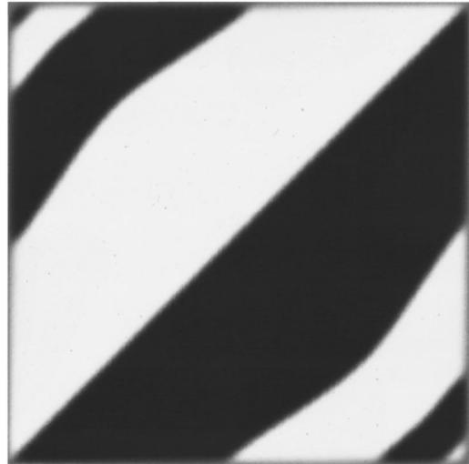
FIG. 1. Grayscale contour plot of the deviatoric strain  $e_2$  for the ground state of a square-columnar grain with sides parallel to T 100-type planes. The black  $\rightarrow$  white range is  $-2.20 \times 10^{-3} \rightarrow +2.20 \times 10^{-3}$ .
