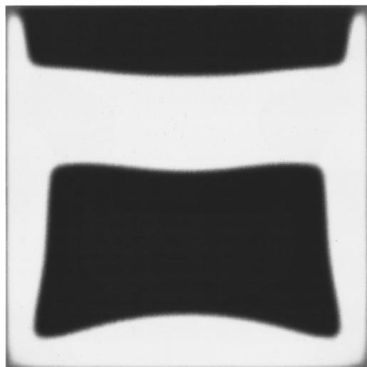
FIG. 2. Grayscale contour plot of the deviatoric strain  $e_2$  for the ground state of a square-columnar grain with sides parallel to T 110-type planes. The black  $\rightarrow$  white range is  $-2.21 \times 10^{-3} \rightarrow +2.20 \times 10^{-3}$ .
