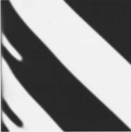
FIG. 5. Tip splitting at the collision of twin walls with a fixed boundary at  $45^\circ$ . The figure gives a grayscale contour plot of the deviatoric strain  $e_2$  for the ground state; the edges are parallel to T 100-type planes.
