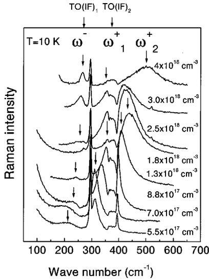
FIG. 1. The Raman spectra of the doped  $(\text{GaAs})_{17}(\text{AlAs})_2$  superlattices. The calculated frequencies of the TO GaAs-like and AlAs-like interface modes are shown at the top of the figure.
