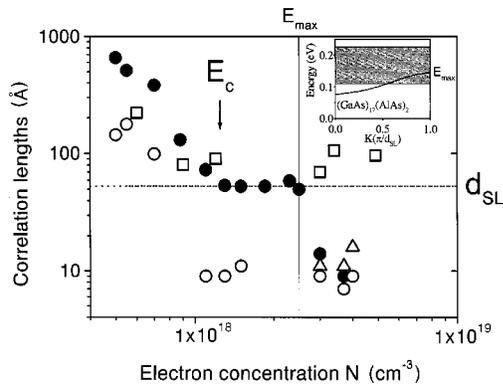
FIG. 4. The coherence lengths  $L$  (open triangles),  $L_1$  (open circles),  $L_2$  (closed circles) of the plasmon-LO phonon excitations  $\omega^-, \omega_1^+, \omega_2^+$  respectively measured in the doped  $(\text{GaAs})_{17}(\text{AlAs})_2$  superlattices with different electron concentrations.  $E_c$  is the mobility edge energy,  $d_{SL}$  is the superlattice period. The squares present the coherence lengths obtained in the doped  $\text{Al}_{0.11}\text{Ga}_{0.89}\text{As}$  alloy.
