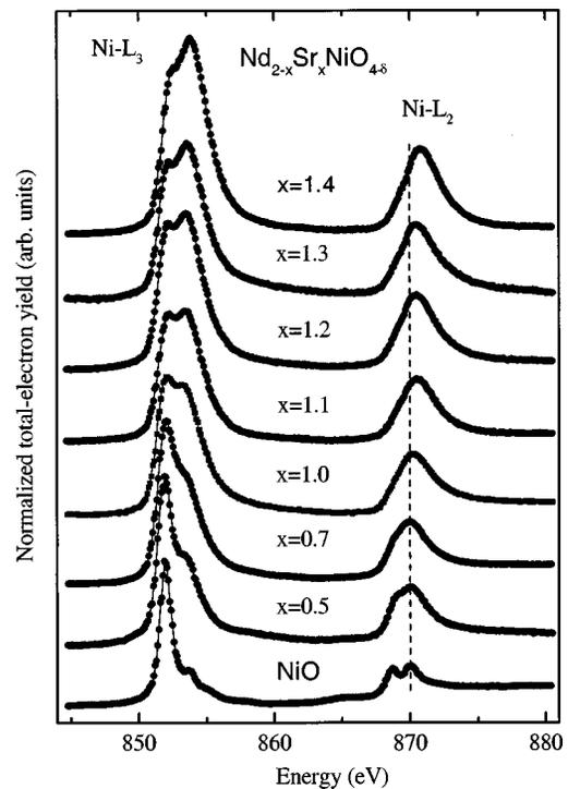
FIG. 3. Ni- $L_{2,3}$  XAS spectra of  $\text{Nd}_{2-x}\text{Sr}_x\text{NiO}_{4-\delta}$  together with data from NiO as reference. The data were recorded using the TY method. The solid curves through the data points serve as a guide to the eyes.
