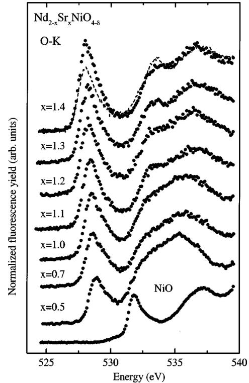
FIG. 1. O-K XAS spectra of  $\text{Nd}_{2-x}\text{Sr}_x\text{NiO}_{4-\delta}$  together with that of NiO as reference. The data were recorded using the bulk-sensitive FY method (filled circles). For comparison, the spectrum obtained for the  $x=1.4$  sample in the TY mode (dashed curve) is also given by the solid line. The solid curves through the data points serve as a guide to the eyes.
