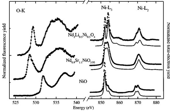
FIG. 4. O-K XAS (left panel) and Ni- $L_{2,3}$  XAS (right panel) spectra of the two formally trivalent Ni oxides,  $\text{Nd}_{0.9}\text{Sr}_{1.1}\text{NiO}_{3.95}$  and  $\text{Nd}_2\text{Li}_{0.5}\text{Ni}_{0.5}\text{O}_4$ , together with NiO as reference. In the right panel, the solid curves below the data points are the results of charge-transfer atomic-multiplet calculations as described in the text.
