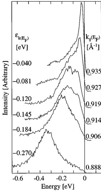
FIG. 2. Photoemission spectra at fixed angle, intensity vs energy. Non-quasiparticle structure is visible in the three spectra with largest momenta. The Fermi momentum is  $0.943 \text{ \AA}^{-1}$ . The momenta and  $\epsilon_k$  quoted are calculated at the Fermi energy and vary slightly across each spectrum. The functional form chosen for  $\epsilon_k$  is discussed in the text.
