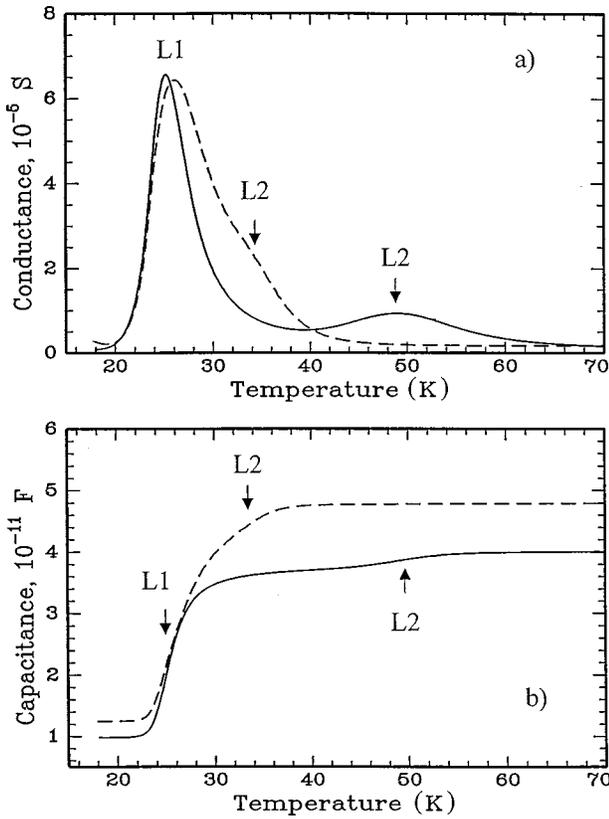
FIG. 1. ADSPEC (a) and TSCAP (b) spectra of the relaxed  $\text{Si}_{1-x}\text{Ge}_x$  layers with  $x=0.05$  (dashed curve) and  $0.1$  (solid curve).
