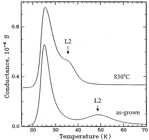
FIG. 3. ADSPEC spectra of the relaxed  $\text{Si}_{1-x}\text{Ge}_x$  layers with  $x=0.1$  before and after annealing at  $850^\circ\text{C}$  for 14 h.
