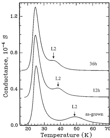
FIG. 2. ADSPEC spectra of the relaxed  $\text{Si}_{1-x}\text{Ge}_x$  layers with  $x=0.1$  annealed at  $470^\circ\text{C}$  for different times.
