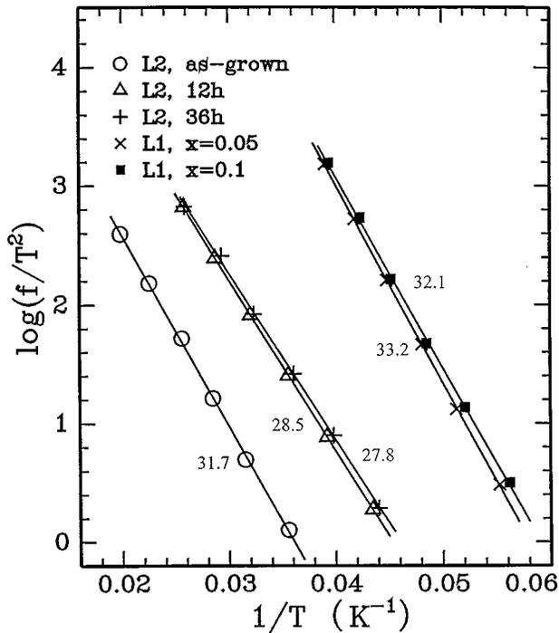
FIG. 4. Arrhenius plots for the level  $L1$  in the samples with  $x = 0.05$  and  $0.1$  and for the level  $L2$  in the sample with  $x = 0.1$ . The plots were deduced from the TSCAP measurements.
