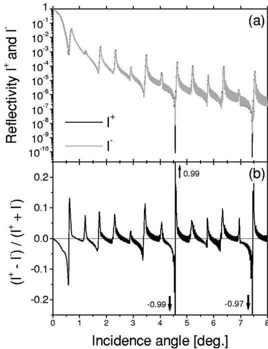
FIG. 4. Calculated resonant reflection of circularly polarized x-rays from Gd/Fe multilayer at the Gd  $L_{III}$  edge (7.243 keV). (a): the reflectivity curves  $I^+$  and  $I^-$  for the clockwise and counterclockwise incident polarizations respectively; (b): their normalized difference. In (a) the difference between the two cases is not appreciable, but in (b) the normalized difference is well seen to vary at the level of about  $\pm 10\%$ .
