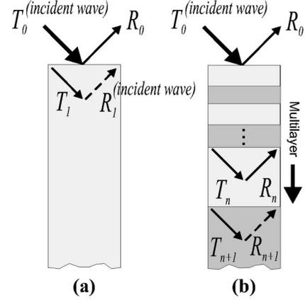
FIG. 2. Schematic illustrating the derivation of matrix recursion equations for x-ray resonant reflection in the cases of (a) a single layer and (b) a multilayer.  $T_k$  and  $R_k$  denote the two-component vectors containing the amplitudes of transmitted and reflected waves, respectively.
