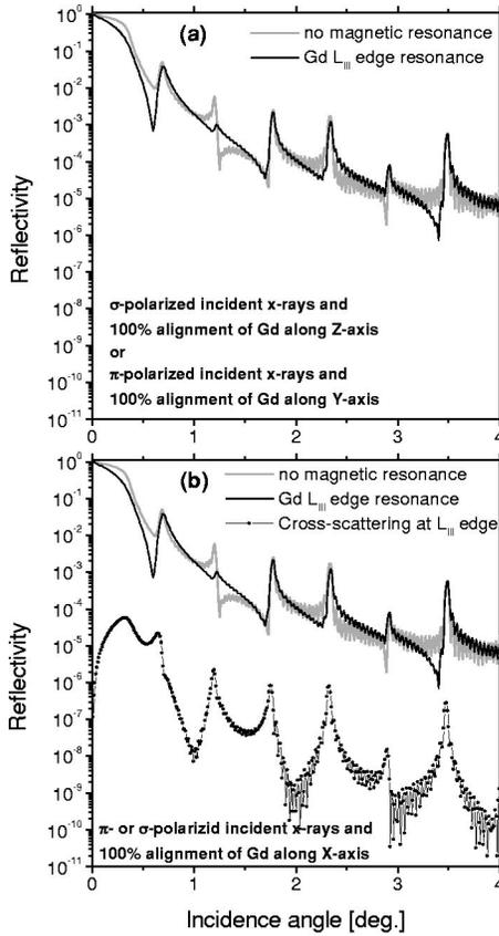
FIG. 3. Calculated resonant reflection of linearly polarized x rays from Gd/Fe multilayer at the Gd  $L_{III}$  edge (7.243 keV) for different directions of the magnetization and incident polarization.
