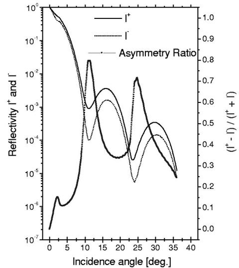
FIG. 5. The calculations of  $I^+$  and  $I^-$  for the case presented in Ref. 30. The sample consists of 36-Å  $\text{Al}_2\text{O}_3$ , 39-Å Co, 5-Å Fe, and 560-Å ZnSe on GaAs substrate; the x-ray energy corresponds to the Co  $L_{III}$  edge (0.7865 keV).
