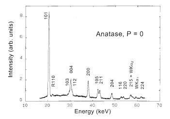
FIG. 1. Energy-dispersive powder-diffraction spectrum of  ${\rm TiO_2}$  at ambient pressure. Miller indices for the Bragg peaks are indicated. The Bragg angle is  $\theta{=}4.95^{\circ}$ . Intensities are given in arbitrary units. The peak denoted R110 is due to a small amount of rutile in the sample.
