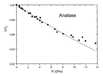
FIG. 4. Relative volume of anatase TiO<sub>2</sub>. Circles and squares denote two experimental runs with polycrystalline anatase, triangles denote single-crystal data, and the solid curve is the result of the theoretical calculation using the *ab initio* perturbed ion model.
