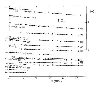
FIG. 2. Lattice plane spacing, d, obtained from powder diffraction, as a function of pressure, P. Circles denote anatase, triangles the baddeleyite phase, and squares the  $\alpha$ -PbO<sub>2</sub> phase. Filled symbols and full lines denote data obtained in a compression run, open symbols and broken lines denote decompression.
