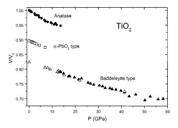
FIG. 3. Experimental pressure-volume data for the polycrystal-line  ${\rm TiO_2}$  polymorphs investigated in the present work. The notation is the same as in Fig. 2. The unit-cell volumes have been normalized by dividing with  $V_{0,\rm anatase}$ .
