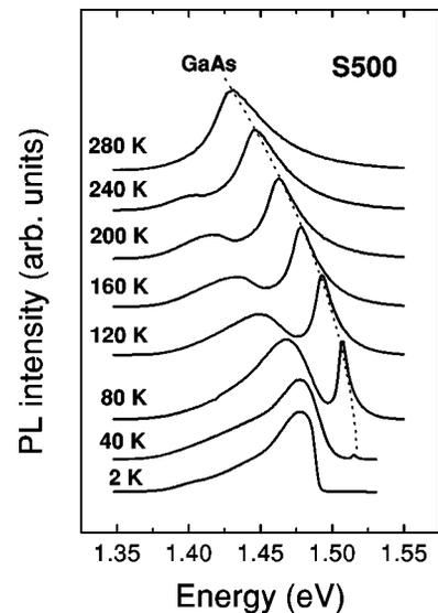
FIG. 2. PL spectra of sample S500 as a function of temperature.
