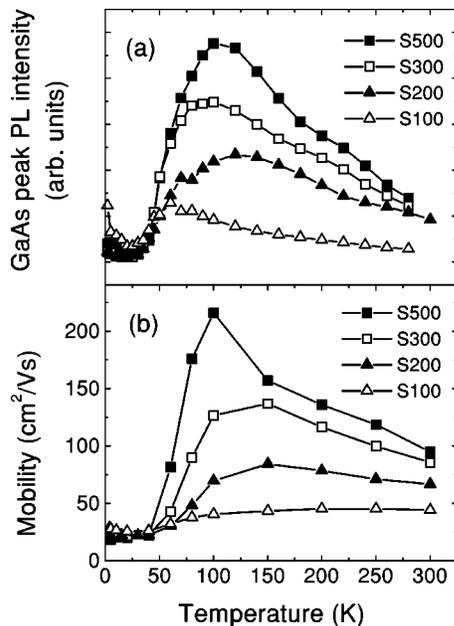
FIG. 6. Temperature dependence: (a) of the absolute maximum intensity of the emission near the GaAs band edge and (b) of the Hall mobility for samples S500, S300, S200, and S100. The lines connecting the points are only a guide to the eyes.
