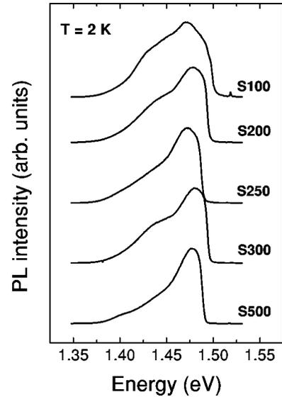
FIG. 1. 2 K PL spectra of multiple  $p$ -type  $\delta$ -doped GaAs layers with a fixed nominal sheet concentration in the  $\delta$ -doped layers ( $N_A = 1.5 \times 10^{13} \text{ cm}^{-2}$ ) and different doping periods  $d$  ranging from 100 to 500  $\text{\AA}$ .
