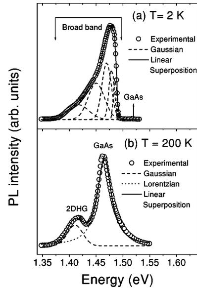
FIG. 4. Representative decomposition of the PL spectra obtained with our line-shape analysis for sample S500 at two different temperatures: (a)  $T=2$  K; (b)  $T=200$  K. The open circles are the experimental data and the solid line represents the linear superposition of the fitted peaks. The vertical arrow in (a) indicates the energy position of the weak GaAs emission.
