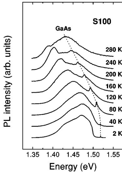
FIG. 5. PL spectra of sample S100 as a function of temperature.
