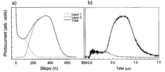
FIG. 2. (a) Simulated photocurrent for a double layer of thickness 30|120 sites and mobility rate  $\mu_1/\mu_2=5/9$ . (b) Experimental photocurrent for a 0.9  $\mu\text{m}$ |9.6  $\mu\text{m}$  organic-organic bilayer with mobility rate of  $\mu_1/\mu_2\sim 1/6$ .
