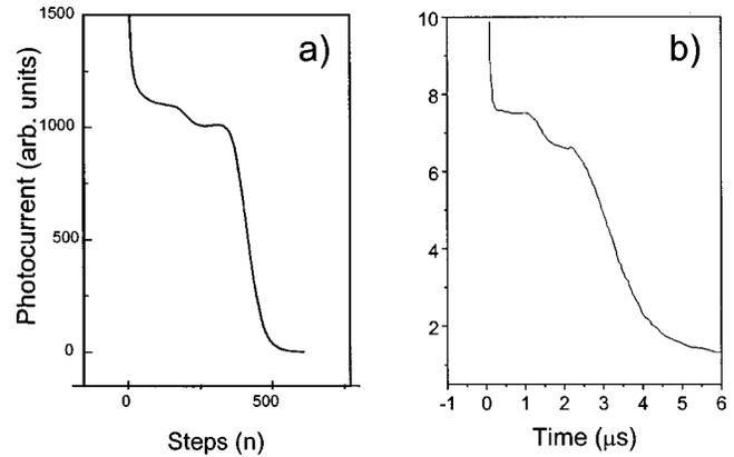
FIG. 5. (a) Simulated photocurrent for a bilayer with a time delay of charge at the interface. The mobility rate was  $\mu_1/\mu_2=1$  and  $t_1=150$  and  $t_2=10$  for  $\phi(t)$ . (b) Experimental photocurrent for an organic-organic bilayer with mobility rate  $\mu_1/\mu_2 \sim 1$  and energy mismatch of approximately 0.13 eV.
