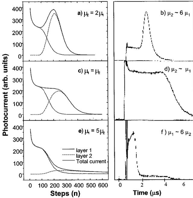
FIG. 1. Simulated photocurrents for a double-layer system with mobility rate of (a)  $\mu_1/\mu_2=5/9$ , (c)  $\mu_1/\mu_2=1$ , and (e)  $\mu_1/\mu_2=5$ , and the experimental counterpart for similar cases with mobility rates of (b)  $\mu_1/\mu_2\sim 1/6$ , (d)  $\mu_1/\mu_2\sim 1$ , and (f)  $\mu_1/\mu_2\sim 6$ . Experimental data were taken from Ref. 2.
