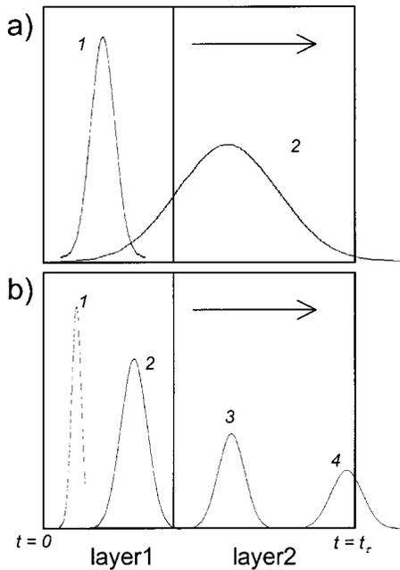
FIG. 3. Representative picture of a packet of particles moving inside a bilayer. (a) The packet can cross continuously the entire sample or (b) cross the layers one by one.
