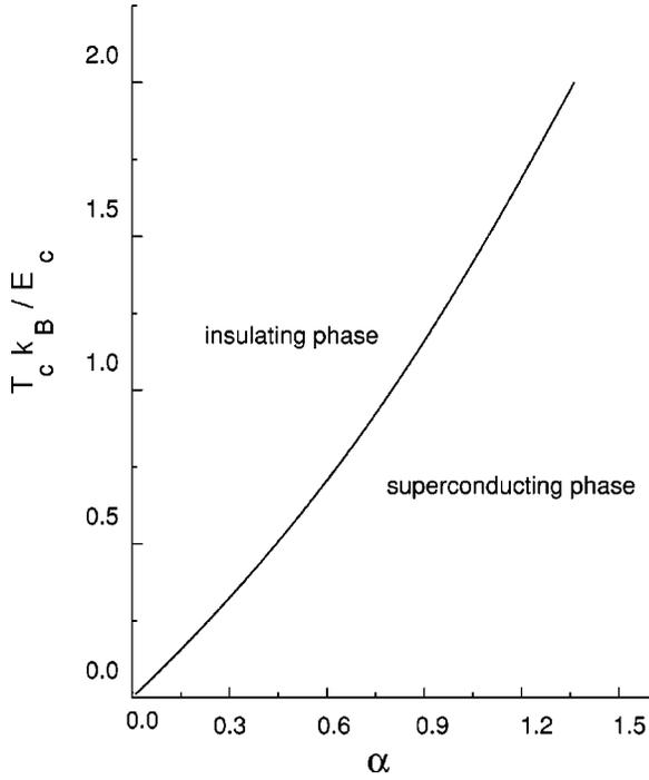
FIG. 2. Phase diagram of the diagonal model with half-integer charge frustration.
