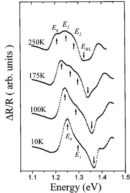
FIG. 4. The EFR spectra of a QD sample at different temperatures. The EFR were measured at  $V_0=0$  V and  $V_b=-4.6$  V.
