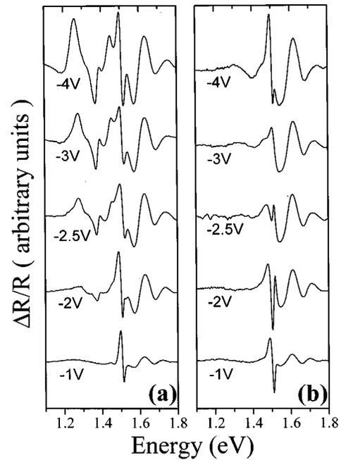
FIG. 2. EFR spectra of (a) QD and (b) referent samples at different reversed biases measured at 10 K.
