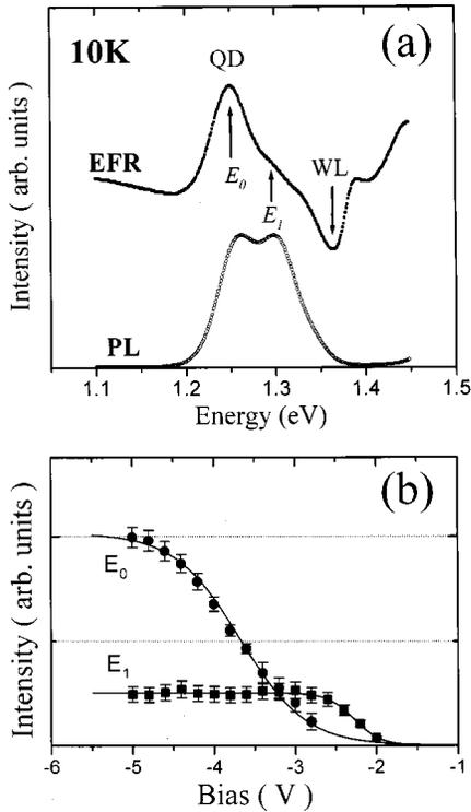
FIG. 3. (a) Comparison of EFR and PL spectra for a QD sample at 10 K. The EFR was measured at  $V_0=0$  V and  $V_b=-4.6$  V. (b) A plot of bias dependent transition intensities of the ground ( $E_0$ ) and first excited ( $E_1$ ) state. The lines are guides for the eye.
