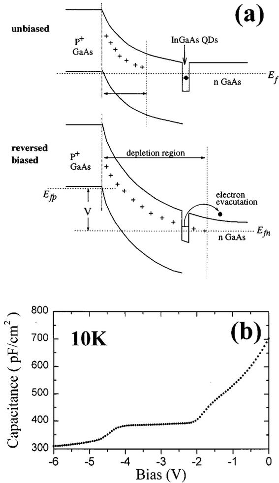
FIG. 1. (a) Schematic diagram of the electron-filling modulation mechanism for quantum dots. (b) Capacitance spectrum of dot samples measured at 10 K.
