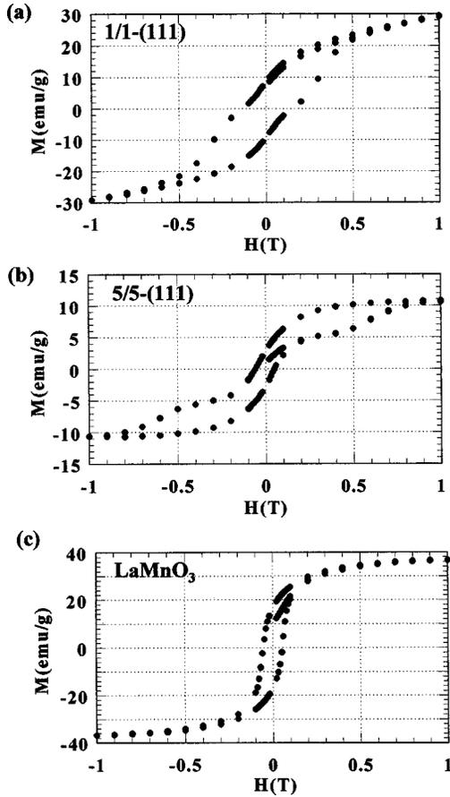
FIG. 3. Hysteresis curves of  $\text{LaMnO}_3\text{-LaFeO}_3$  superlattices formed on  $\text{SrTiO}_3$  (111) with (a) 1/1 and (b) 5/5 stacking periodicity, and (c) that of the  $\text{LaMnO}_3$  film at 6 K.
