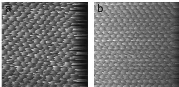
FIG. 3. Atomic stick-slip behavior of the lateral force measured on a Cu(111) surface. Dark corresponds to low forces, bright to high forces. Two different spring constants were used: (a) Image size 3 nm×3 nm,  $k_n=0.01$  N/m. (b) Image size 3.5 nm×3.5 nm,  $k_n=24$  N/m.
