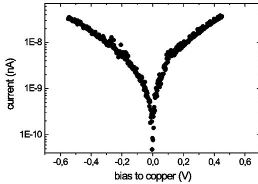
FIG. 2. I-V-characteristic of the tip in contact with the sample. The absolute value of the current is given in a logarithmic scale.
