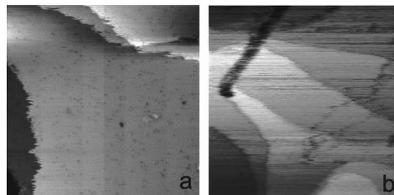
FIG. 1. Overview images of the Cu(111) surface. (a) Image taken in the STM mode ( $92 \text{ nm} \times 92 \text{ nm}$ ), showing terraces of 50–250 nm width, separated by monatomic steps. The black dots represent single atom sulfur impurities. (b) Contact-mode force microscopy image ( $114 \text{ nm} \times 114 \text{ nm}$ ) of the same sample.
