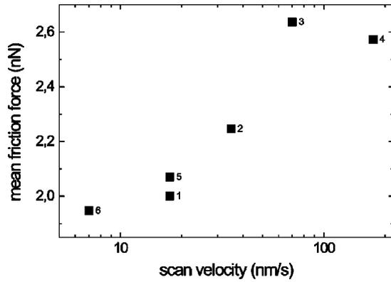
FIG. 5. Velocity dependence of atomic-scale friction on Cu(111). The labels indicate the temporal order of measurement.
