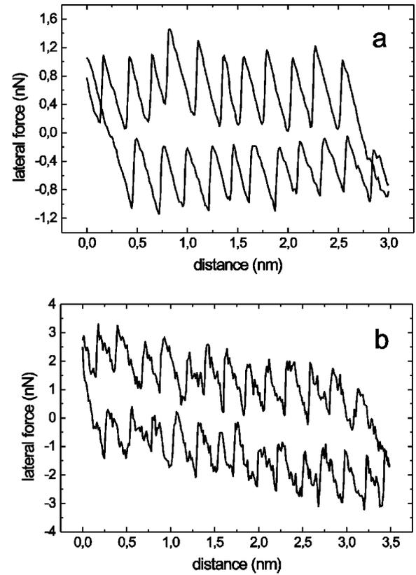
FIG. 4. Lateral force along a (110) direction. Two different spring constants were used: (a)  $k_n=0.01$  N/m. (b)  $k_n=24$  N/m.
