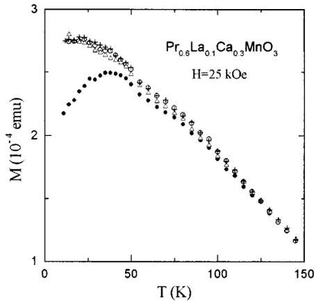
FIG. 3. Temperature dependences of magnetization measured in the field  $H = 25$  kOe in the unilluminated film (full and open circles show ZFC and FC dependences, respectively) and in the film under illumination (crosses and triangles show ZFC and FC dependences, respectively).
