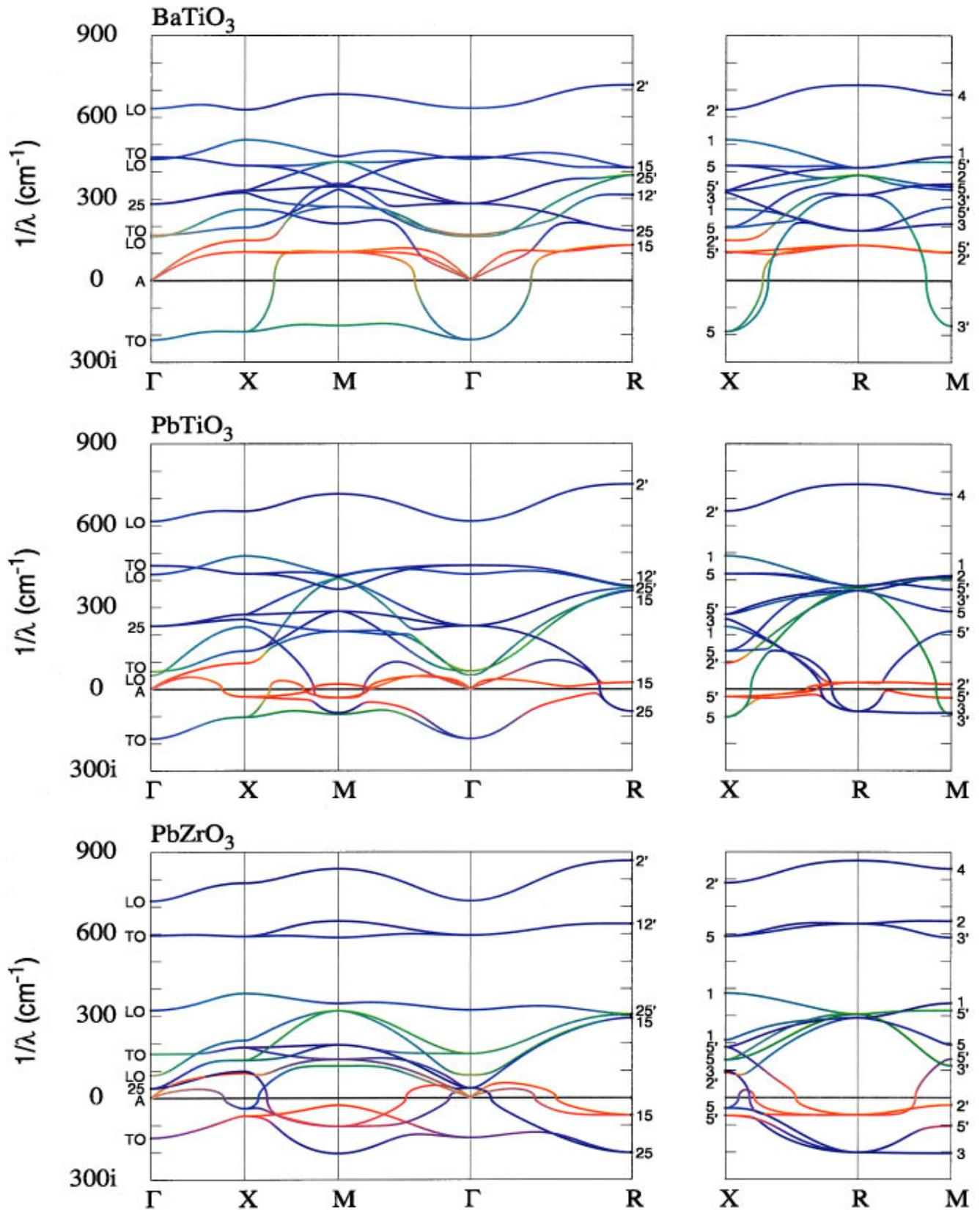
FIG. 1. (Color) Calculated phonon dispersion relations of BaTiO<sub>3</sub>, PbTiO<sub>3</sub>, and PbZrO<sub>3</sub> along various high-symmetry lines in the simple cubic Brillouin zone. A color has been assigned to each point based on the contribution of each kind of atom to the associated dynamical matrix eigenvector (red for the A atom, green for the B atom, and blue for the oxygens) (Ref. 35). Symmetry labels follow the convention of Ref. 40, with the A atom at the origin.
