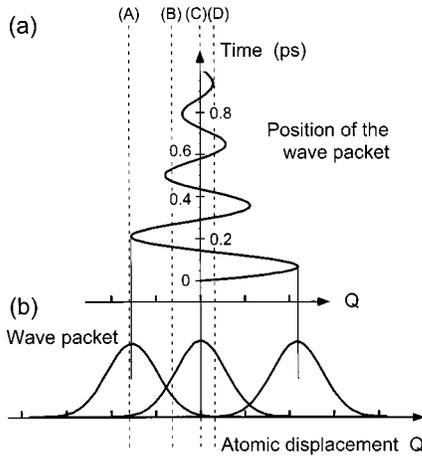
FIG. 4. (a) Time development of the central position of the wave packet,  $Q_c(t)$ , assumed in the calculation. (b) Gaussian-shaped wave packet assumed in the calculation. The scale of the  $Q$  axis is exactly the same as that in Fig. 3.
