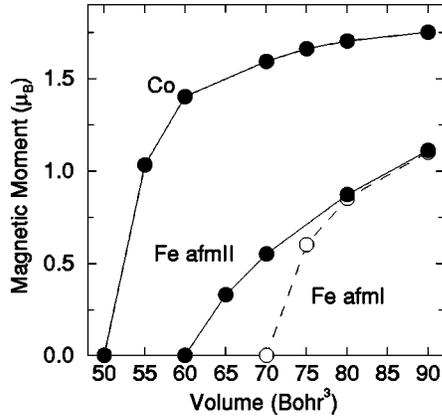
FIG. 1. Magnetic moment per atom within the muffin-tin sphere for the two antiferromagnetic states of iron considered here and the ferromagnetic moment for cobalt as a function of volume.
