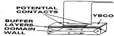
FIG. 2. Diagram of sample with four electrical contacts to the superconductive film and leads used to measure ac voltages. Domains of magnetization  $\mathbf{M}$  are shown within the Ni RABiTS.
