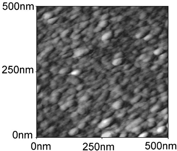
FIG. 1. AFM image of Fe layer. The image shows elongated Fe grains with the mean length and width as  $36 \pm 12$  nm and  $21 \pm 7$  nm, respectively. Note that the major axes are all parallel.
