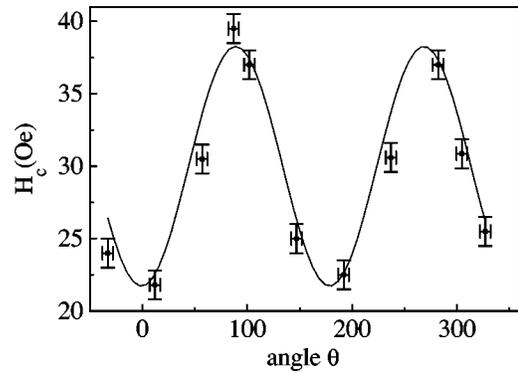
FIG. 2. Measurements of coercive field ( $H_C$ ) by changing the angle between the magnetic anisotropy axis and the magnetic field applied in the plane of the film. This curve indicates that the magnetic anisotropy is uniaxial. The line is a guide to the eyes.
