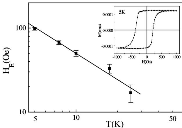
FIG. 4. Exchange bias field ( $H_E$ ) as a function of temperature in log-log scale. The inset shows a hysteresis loop performed at 5 K, shifted to negative fields.
