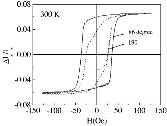
FIG. 3. Hysteresis loop for  $\theta=86$  (full line) and  $190^\circ$  (dashed line) measured by MOKE at 300 K.
