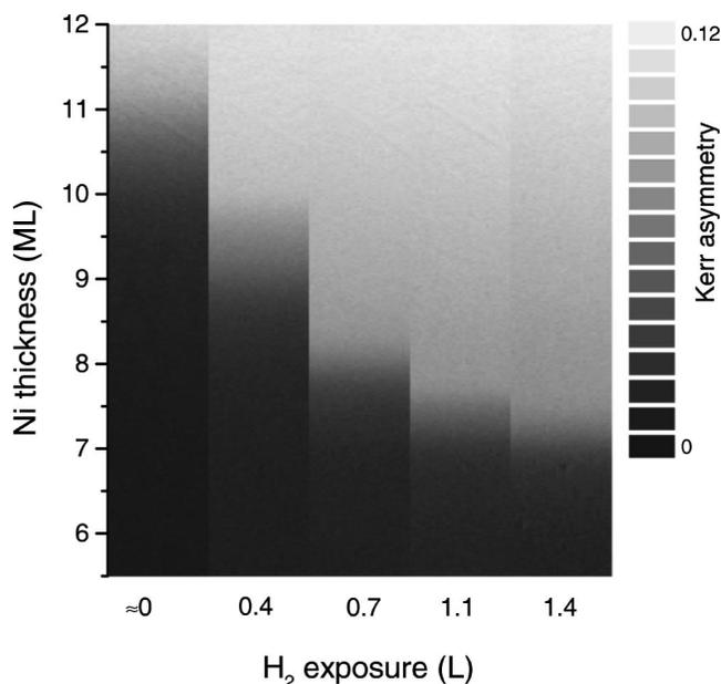
FIG. 2. Polar Kerr asymmetry images of the same section of a Ni wedge on Cu(001) for five  $H_2$  exposures at  $T=143$  K. The Ni thickness increases from the bottom to the top of the image as indicated by the scale on the left hand side. The bright area indicates the presence of perpendicular magnetization, the dark area in-plane magnetization.
