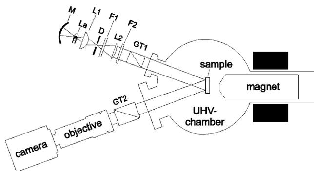
FIG. 1. Schematic view of the experimental Kerr microscopy setup: M, mirror; La, halogen lamp; L1, condenser; D, diaphragm; F1, F2, colored glass filters; L2, lens  $f=100$  mm; GT1, Glan-Thompson polarizer; GT2, analyzer (Glan-Thompson).
