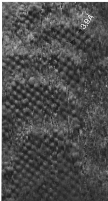
FIG. 8. STM image of a growth spiral taken on top of a ridge of the canyonlike structure of Fig. 6.
