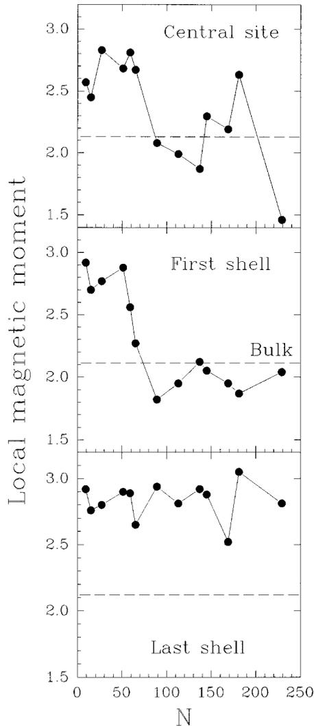
FIG. 4. Magnetic moments (in units of  $\mu_B$ ) of the central site (upper panel), first shell (central panel), and last outer shell (lower panel) as a function of the cluster size.
