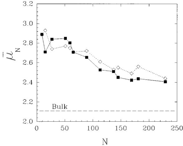
FIG. 2. Average magnetic moment per atom (in units of  $\mu_B$ ) obtained with our model (black squares) and by Guevara *et al.* (Ref. 19) considering the electronic spillover (open rhombus).
