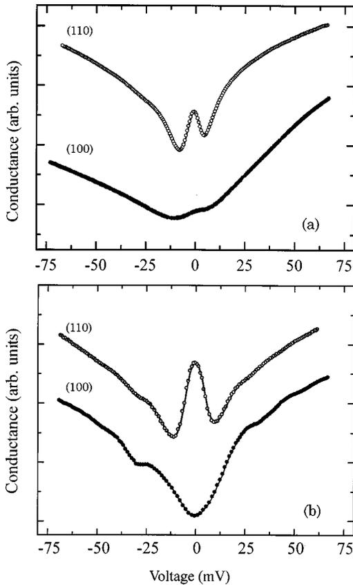
FIG. 3. Typical conductance vs voltage curve for the (110) and (100) junction fabricated on the same substrate.
