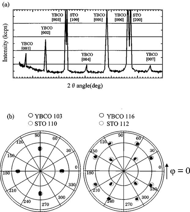
FIG. 1. (a) XRD pattern of the YBCO thin film grown on  $\text{SrTiO}_3$  substrate. (b), (c): Pole figure of the YBCO thin film observed at the detection angles  $2\theta$  of  $32.84^\circ$  and  $58.20^\circ$ , respectively.
