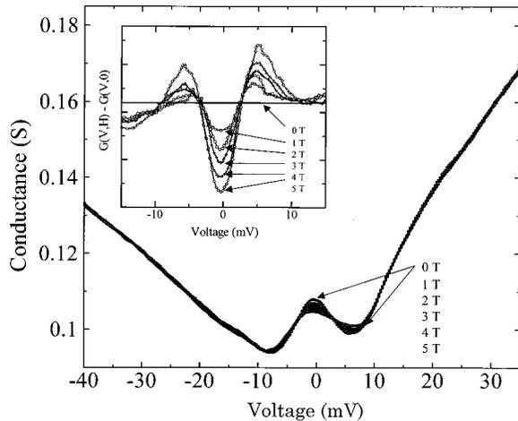
FIG. 5. Magnetic-field dependence of the conductance for a (110) junction at 4.2 K. The inset shows the relationship between  $G(V,H)-G(V,0)$  and bias voltage  $V$ .
