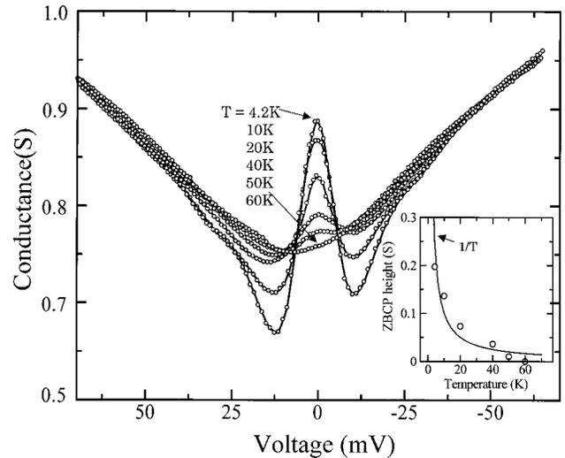
FIG. 4. Conductance vs voltage curves measured at different bath temperatures. The inset shows the temperature dependence of the zero-bias peak height for a (110) junction.
