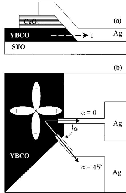
FIG. 2. (a) Schematic cross-sectional view of ramp-edge junction. (b) Two ramp-edge junctions fabricated on one STO substrate with tilted angles of  $45^\circ$  and  $0^\circ$  against the  $a$  axis of YBCO film.
