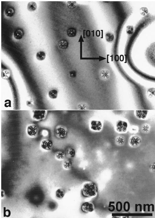
FIG. 1. Plan-view [001] on-zone bright-field images of (a) sample A and (b) sample B.
