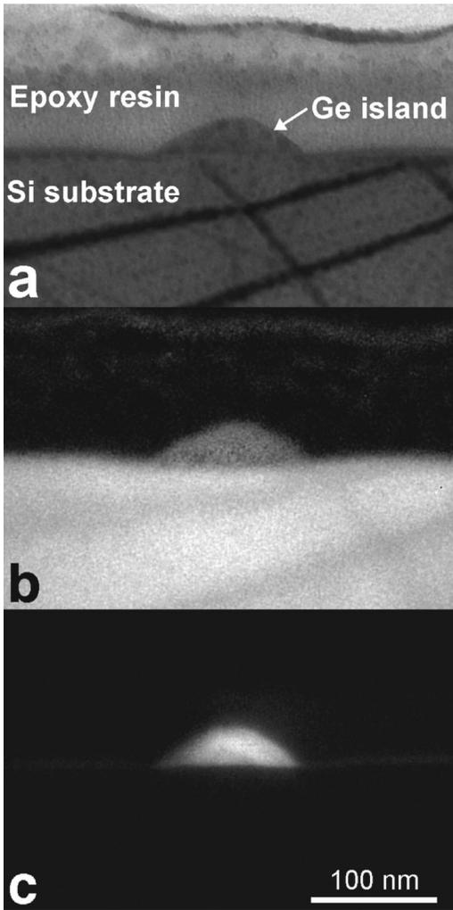
FIG. 3. Cross-section energy-filtered images: (a) a zero-loss image showing the complete morphology of the TEM specimen; (b) an energy-loss (1839 eV) image that represents a Si map. Si is clearly seen within the island; and (c) an energy-loss (1217 eV) image that represents a Ge map. A wetting layer is seen uniformly throughout the entire substrate surface.
