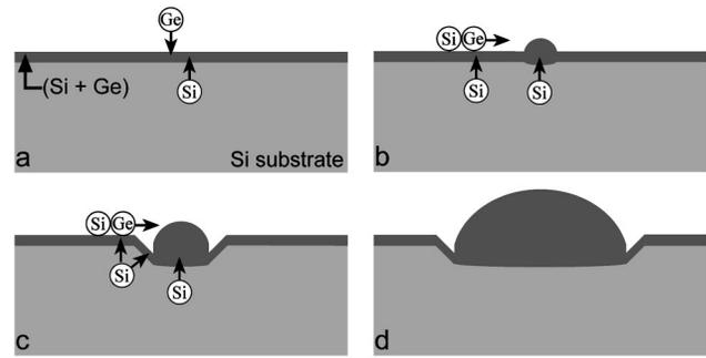
FIG. 4. Schematic diagrams of a modified S-K growth mode at different growth stages.
