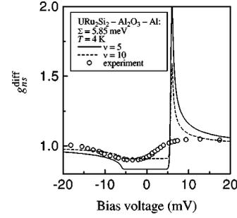
FIG. 5. Dependences  $g_{ns}^{diff}(V)$  for the ns junction  $URu_2Si_2$ - $Al_2O_3$ - $Al$  in the normal state taken from the experiment (Ref. 46) and calculated for various  $\nu$ 's.
