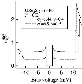
FIG. 4. Conductances  $g_{ns}^{diff}(V)$  of the  $URu_2Si_2$ - $I$ - $Pb$  junction for the sets of parameters from Ref. 29 (solid curve) and Ref. 30 (dashed curve).
