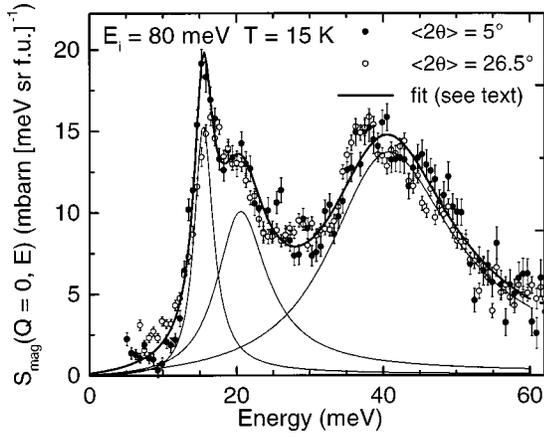
FIG. 3. Magnetic energy spectra of  $\text{YbB}_{12}$  at  $T=15$  K, measured with the incident neutron energy  $E_i=80$  meV, for two different scattering angles. Intensities have been scaled to  $Q=0$  using the  $\text{Yb}^{3+}$  form factor. Lines represent a fit to a spectral function consisting of three Lorentzian peaks.
