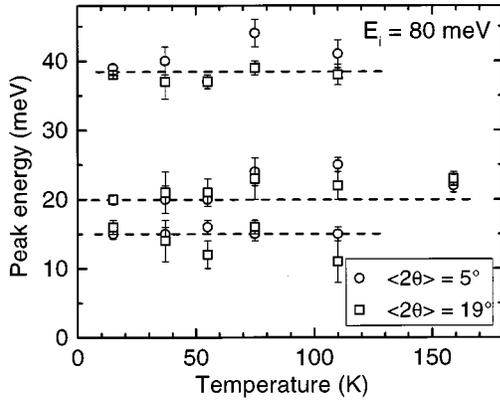
FIG. 6. Temperature dependence of the magnetic peak positions in  $\text{YbB}_{12}$  in spectra measured for two different scattering angles. The values for  $\langle 2\theta \rangle \approx 19^\circ$  were obtained by averaging the spectra over the angular range  $11^\circ \leq 2\theta \leq 26.5^\circ$  prior to fitting. The dashed lines correspond to the constant energies  $E = 15, 20,$  and  $38 \text{ meV}$ .
