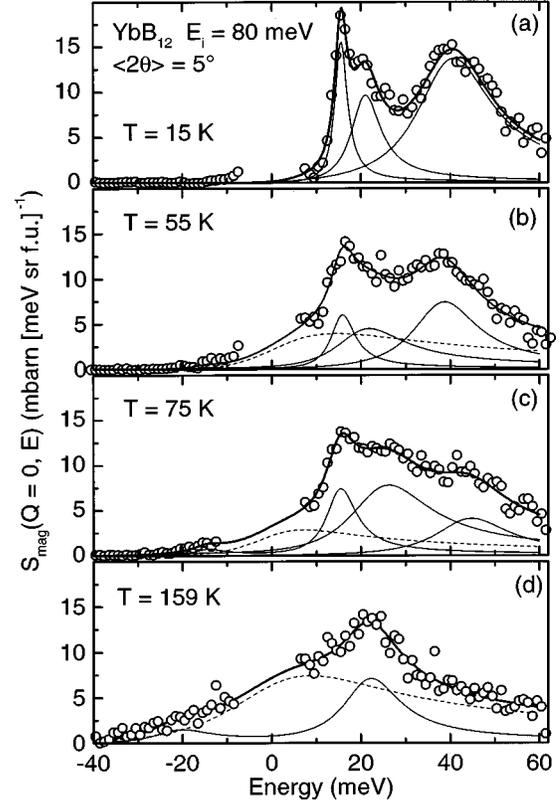
FIG. 5. Magnetic energy spectra,  $S_{\text{mag}}(Q=0, E)$ , of  $\text{YbB}_{12}$  at four different temperatures, measured at the lowest scattering angle  $\langle 2\theta \rangle = 5^\circ$  with the incident energy  $E_i=80$  meV. The lines represent a fit to a spectral function consisting of inelastic (thin lines) and quasielastic (dashed line) Lorentzian peaks.
