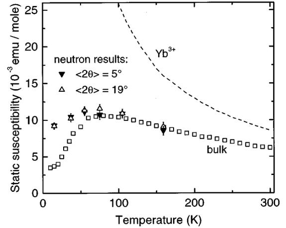
FIG. 8. Temperature dependence of the static magnetic susceptibility.  $\Delta$ ,  $\blacktriangledown$ : data derived from the neutron spectra for two different average scattering angles (error bars denote the estimated uncertainty in the absolute normalization of the data);  $\square$ : bulk susceptibility from Ref. 2; dashed line: static susceptibility calculated as  $\chi_{\text{st}}(T) = p_{\text{loc}}^2 \mu_B^2 / 3k_B T$ , with  $p_{\text{loc}} = 4.54$  for  $\text{Yb}^{3+}$ .
