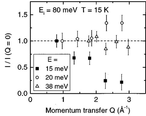
FIG. 4. Normalized  $Q$  dependence of the integrated intensities of the different magnetic spectral components of  $\text{YbB}_{12}$  at  $T=15$  K (incident energy  $E_i=80$  meV).
