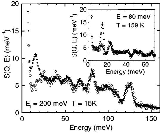
FIG. 1. Energy spectra of  $\text{LuB}_{12}$  (open circles) and  $\text{YbB}_{12}$  (black dots) at  $T=15$  K, measured with the incident neutron energy  $E_i=200$  meV at a scattering angle  $\langle 2\theta \rangle=130^\circ$ . The spectra are normalized with respect to the intensity of the peak at 125 meV. Inset: energy spectra at  $T=159$  K for  $\langle 2\theta \rangle=130^\circ$  and  $E_i=80$  meV; the two spectra have been normalized in the high-energy region ( $E=60-70$  meV).
