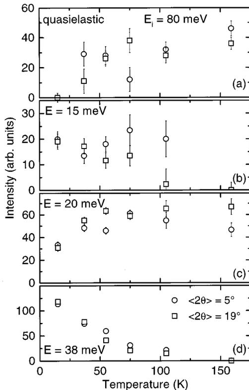
FIG. 7. Temperature dependence of the integrated intensities for (a) the quasielastic peak, and the inelastic peaks at (b) 15, (c) 20, and (d) 38 meV. Two sets of points correspond to different average scattering angles and different resolution conditions.
