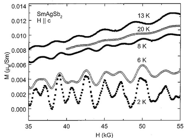
FIG. 6. Magnetization as a function of applied field in  $\text{SmAgSb}_2$  up to 20 K.
