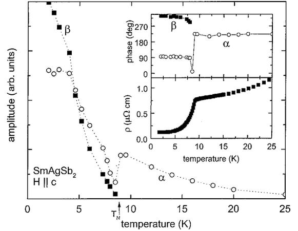
FIG. 8. Temperature dependence of the amplitudes of the  $\alpha$  and  $\beta$  oscillations in  $\text{SmAgSb}_2$ . Top inset: temperature dependence of the relative phase of the oscillations. Bottom inset: temperature dependence of the resistivity. Note the suppression of the  $\alpha$  amplitude and discontinuity in the phase at  $T_N = 8.8$  K.
