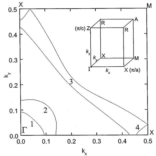
FIG. 10. The Fermi surface of LaAgSb<sub>2</sub> in the  $k_z=0$  plane, calculated as described in the text. The four bands crossing  $E_F$  are labeled 1–4. Inset: the Brillouin zone of a primitive tetragonal lattice with the high-symmetry points labeled.
