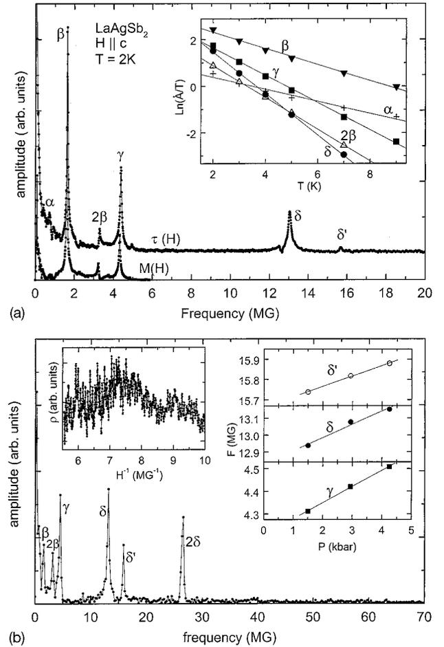
FIG. 3. (a) Fourier spectrum of the oscillations in the torque and magnetization of  $\text{LaAgSb}_2$  for  $H\parallel c$  at 2 K. Inset: Temperature dependence of the amplitudes of the observed oscillations. (b) Fourier spectra of SdH oscillations in  $\text{LaAgSb}_2$  at 4.2 kbars and 2.1 K. Left inset: resistivity as a function of inverse field. Right inset: pressure dependence of the frequencies of the observed oscillations.
