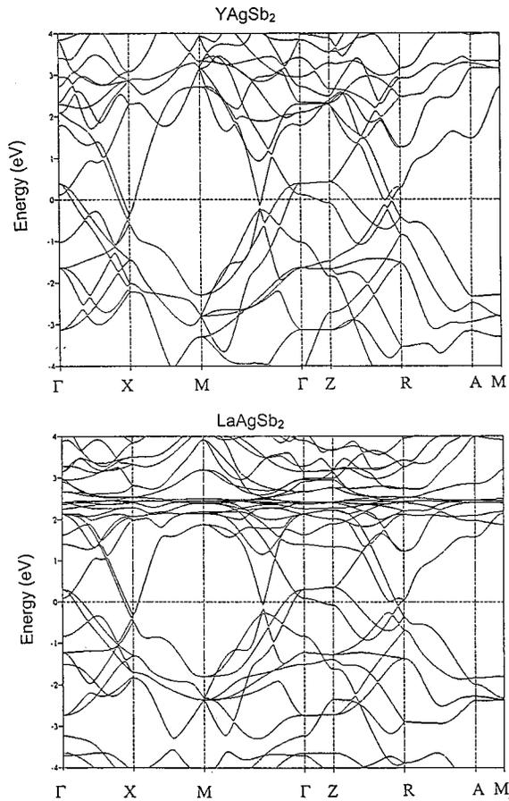
FIG. 9. Band structure of (a) YAgSb<sub>2</sub> and (b) LaAgSb<sub>2</sub> calculated from tight-binding linear muffin-tin orbital calculations within the atomic spheres approximation.
