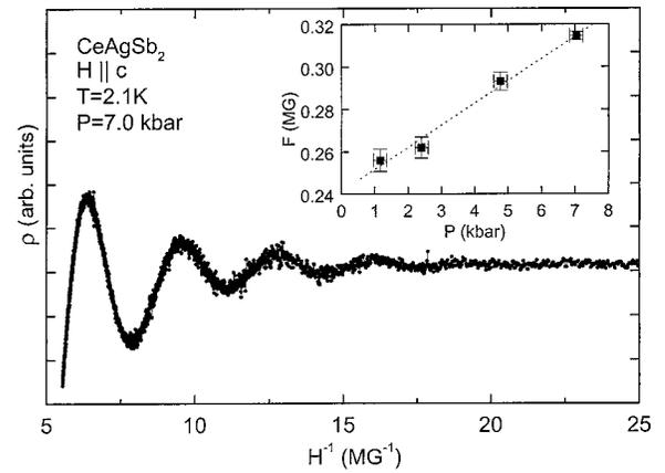
FIG. 5. Shubnikov–de Haas oscillations in  $\text{CeAgSb}_2$  at 2.1 K and 7.0 kbars. The background magnetoresistance has been removed. Inset: pressure dependence of the SdH oscillation.
