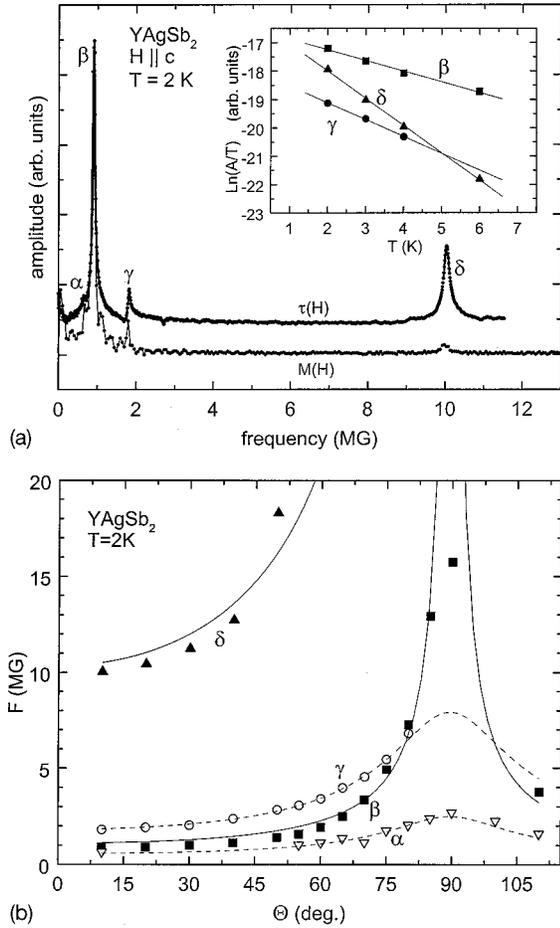
FIG. 2. (a) Fourier spectrum of the oscillations in  $\text{YAgSb}_2$  for  $H\parallel c$  at 2 K. Inset: Temperature dependence of the amplitudes of the observed oscillations. (b) Angular dependence of the frequencies.  $\theta$  is relative to the  $c$  axis. The lines are fits to the cross-sectional areas of a cylinder ( $\beta$  and  $\delta$ ) and an ellipsoid ( $\alpha$  and  $\gamma$ ).
