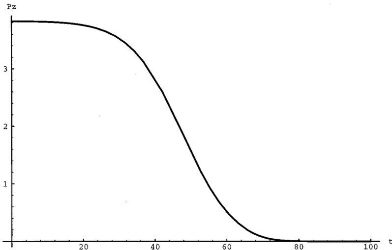
FIG. 10. Some graphical illustrations of the change of the  $z$  component of the total magnetic momentum  $P_z$  expressed by Eq. (56) in a ferromagnet with an easy axis, where  $\rho=0.1$ ,  $k'_1=0.1$ ,  $k''_1=0.2$ ,  $x_{10}=0$ , and  $x_{20}=0$ .
