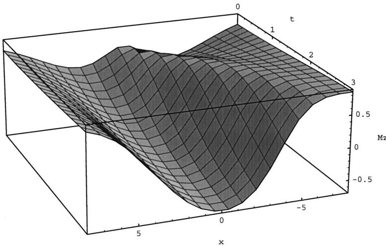
FIG. 7. Some graphical illustrations of the motion of the center and the change of shape of the  $z$  component of the nonlinear magnetization  $(\mathbf{M}_1)_z$  expressed by Eq. (53) in an isotropic ferromagnet, where  $\rho=0$ ,  $k'_1=0.1$ ,  $k''_1=0.2$ ,  $x_{10}=0$ , and  $x_{20}=0$ .
