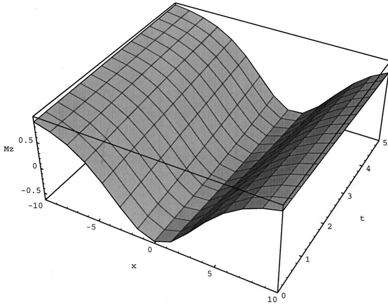
FIG. 5. Some graphical illustrations of the change of amplitude and width of the  $z$  component of the nonlinear magnetization  $(\mathbf{M}_1)_z$  expressed by Eq. (51) in a ferromagnet with an easy plane, where  $\theta_0=30^\circ$ ,  $\rho=0.2$ ,  $k'_1=0.1$ ,  $k''_1=0.2$ ,  $x_{10}=0$ , and  $x_{20}=0$ .
