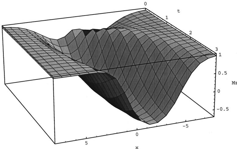
FIG. 4. Some graphical illustrations of the motion of the center and the change of shape of the  $z$  component of the nonlinear magnetization  $(\mathbf{M}_1)_z$  expressed by Eq. (43) in a ferromagnet with an easy axis, where  $\rho=0.3$ ,  $k'_1=0.1$ ,  $k''_1=0.2$ ,  $x_{10}=0$ , and  $x_{20}=0$ .
