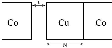
FIG. 1. Schematic representation of a Co/vacuum/Cu/Co tunneling junction, with hopping matrix  $t$  across the vacuum gap.
