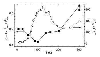
FIG. 4. Temperature dependence of the CL contrast *C* (squares) and the ratio  $R_{PL}^{-1}$  (circles) of the spatially integrated intensities of the Qwire and Qwell CL. The contrast was measured by CL line scans.
