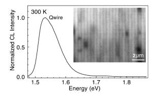
FIG. 2. CL spectrum and CL image of a stacked Qwire array on GaAs(311)A substrate at 300 K. The detection energy is set to the maximum position of the CL spectrum. Note the strong Qwire related CL contrast in the CL micrograph, although the Qwell CL has almost completely disappeared.
