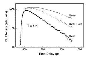
FIG. 6. Time dependence of the PL intensity obtained from the Qwire and Qwell regions of the wire array and from the reference Qwell at 5 K.
