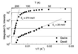
FIG. 5. Temperature dependence of the integrated CL intensities originating from the Qwire (circles) and connecting Qwell (squares) regions. The dashed lines describe an exponential temperature dependence with the respective activation energy  $(E_a)$ .
