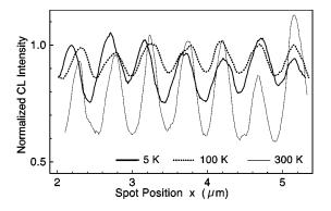
FIG. 3. Normalized CL line profiles perpendicular to the wires of a stacked Qwire array at different temperatures. The respective detection energy is set to the maximum position of the wire line.
