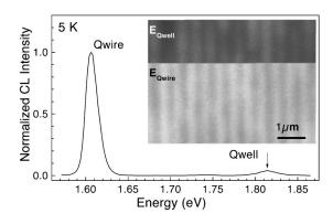
FIG. 1. CL spectrum and CL image of a stacked Qwire array on GaAs(311)A substrate at 5 K. For the upper (lower) part of the CL image, the detection energy was set to the Qwell (Qwire) CL line of the spectrum.
