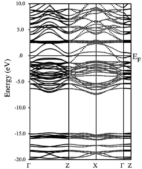
FIG. 2. Band structure of the majority-spin channel of  $\text{LaSr}_2\text{Mn}_2\text{O}_7$ .
