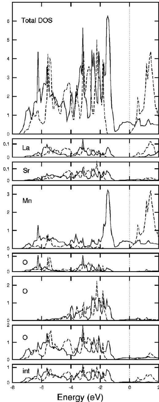
FIG. 4. Total density of states, density of states per atom, and density of states in the interstitial space (in states/eV). The solid (dashed) line denotes the density of states of the majority-(minority-) spin channel. The three different O atoms successively lie in the same layer as the La, Sr, and Mn atoms.
