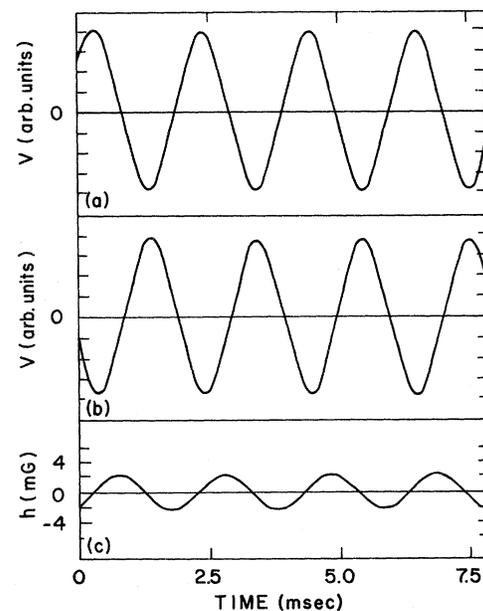
FIG. 3. Induced time-dependent voltage  $V(t)$  at field  $H_0 = 600$  G, where in (a)  $H_0$  was reached from above and in (b)  $H_0$  was reached from below. (c) The modulating magnetic field  $h$  vs time.
