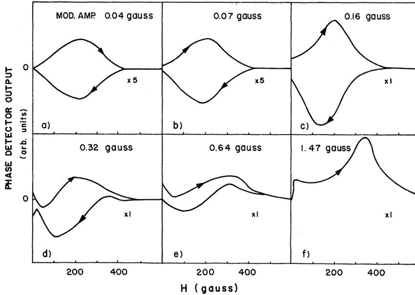
FIG. 5.  $V_0 \sin \delta$  vs  $H$  for several different values of  $h_0$ . (a)  $h_0 = 0.04$  G, (b) 0.07 G, (c) 0.16 G, (d) 0.32 G, (e) 0.64 G, (f) 1.47 G. In (a) and (b)  $V_0$  has been multiplied by a factor of 5.
