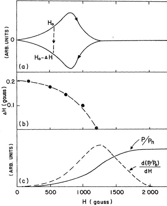
FIG. 4. (a) Phase-sensitive detector output  $V_0 \sin \delta$  vs  $H$ . The dashed line indicates the path in which the phase is reversed by changing the field by an amount  $\Delta H$ . (b) The minimum  $\Delta H$  required to change the phase of  $V(t)$ . (c) Solid line: resistive transition obtained by measuring the microwave absorption. Dashed line: mathematical derivative of the solid line.
