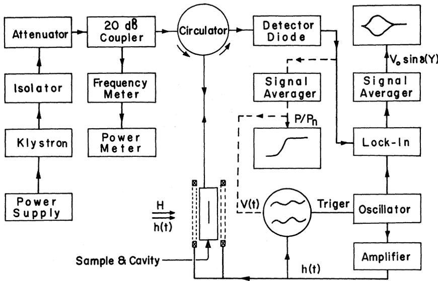
FIG. 2. Block diagram for the microwave electronic system.
