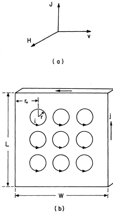
FIG. 1. (a) Vector relation among the external magnetic field  $\vec{H}$ , the microwave current  $\vec{J}$ , and the flux-flow velocity  $\vec{v}$ . (b) Geometry used in the text to estimate the force between the boundary current  $j$  and the flux lattice. The flux lines are represented by ring currents  $i$  of radius  $r$ .  $W$  is the width of the sample along the  $y$ -direction.  $L$  is the length.
