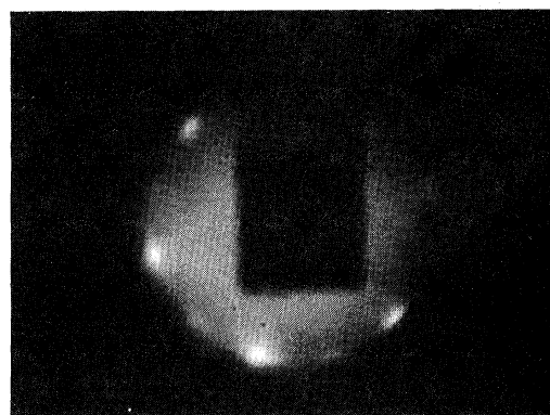
FIG. 2. LEED pattern from the (111) face of neon adsorbed on Nb(100). Dark rectangle in foreground is a cryogenic shield surrounding the sample. Note trace of pseudo-12-fold symmetry.
