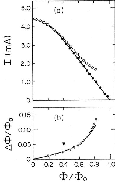
FIG. 5. (a) Maximum current  $I_M$  (solid circles) and  $I'_M = I_1(f_p^4/f_J^4 + I_R^2/I_c^2)^{1/2}$ ,  $f_p = 9.0$  GHz (open circles), as a function of the applied flux. Smooth curves have been fitted to the data. (b) The difference  $\Delta\Phi$  (open triangles) as a function of the applied flux obtained from (a). The line through the data is the function  $\beta I_c$  ( $\beta = 0.0229 \text{ mA}^{-1}$ ). The direct numerical result for  $\Delta\Phi$  is shown as a solid triangle.
