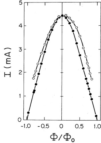
FIG. 3. Maximum dc current  $I_M$  (solid circles) and  $I_1(f_p/f_J)^2[1 - (I_R/I_M)^2]^{-1/2}$ ,  $f_p = 9.0$  GHz (open circles) vs the applied flux  $\Phi_y = \mu_0 H_y L d$ . Smooth curves have been fitted to the data.
