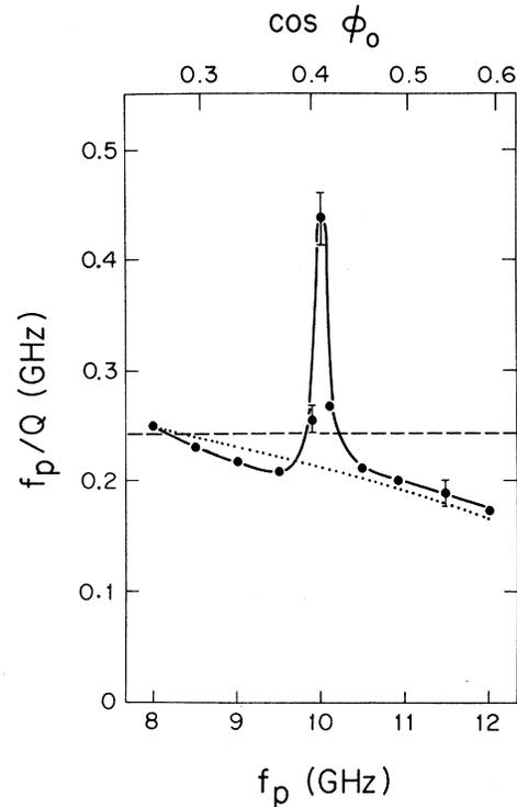
FIG. 7.  $f_p Q^{-1}$  as a function of frequency. A smooth curve has been fitted to the data. The dashed line is  $(2\pi R_N C)^{-1}$ ,  $R_N = 0.46 \Omega$ ,  $C = 1.5$  nF. Typical error bars are shown. See text for discussion of dotted line.
