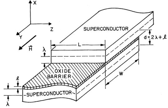
FIG. 1. Junction geometry.
