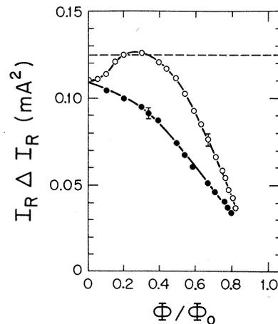
FIG. 8.  $I_R \Delta I_R$  as a function of the applied magnetic flux, open circles for  $\Phi/\Phi_0 > 0$ , solid circles for  $\Phi/\Phi_0 < 0$ . The dashed line is the calculated value of  $I_R \Delta I_R$  obtained using the experimental values of  $f_p$ ,  $R_N$ , and  $C$ . Typical error bars are shown.
