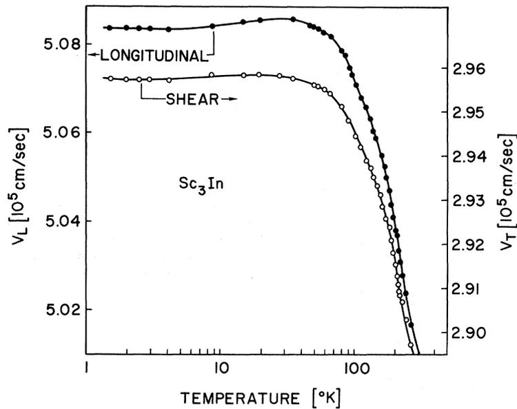
FIG. 3. Temperature dependence of the longitudinal and shear (transverse) velocity of sound in polycrystalline  $\text{Sc}_3\text{In}$ .
