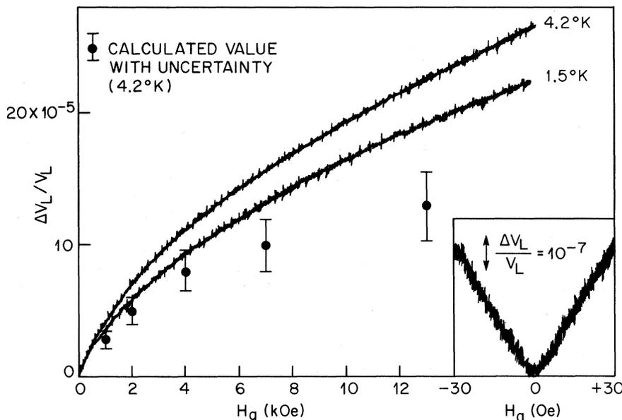
FIG. 4. Fractional change in longitudinal-wave sound velocity (20 MHz) vs applied field for  $\text{Sc}_3\text{In}$ . The insert shows data taken over a small-field range under quieter conditions. The indicated noise is representative. The reproducibility of the data is  $\sim 10\%$ .
