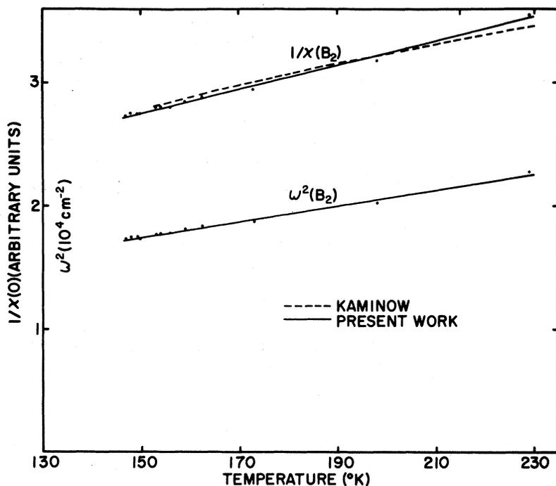
FIG. 2. Temperature dependence of the uncoupled overdamped frequency square  $\omega^2(B_2)$  and the inverse susceptibility  $1/\chi(B_2)$  of the  $B_2$  mode in  $\text{NH}_4\text{H}_2\text{PO}_4$  above the Curie point.
