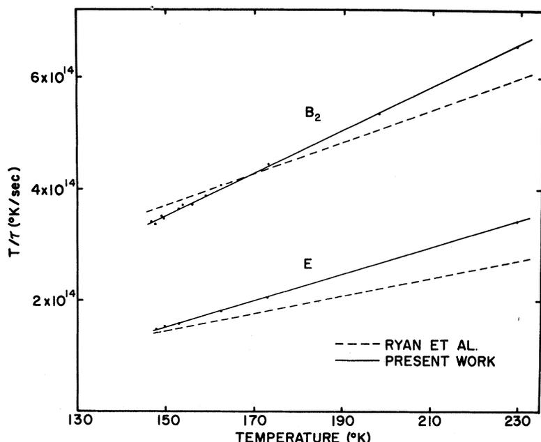
FIG. 3. Temperature dependence of the weighted equivalent inverse relaxation time  $T/\tau$  of  $\text{NH}_4\text{H}_2\text{PO}_4$  for both  $B_2$  and  $E$  overdamped modes above the Curie point.
