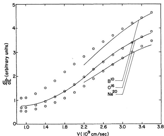
FIG. 5. Calculated values (represented by open circles) of scintillation efficiency versus velocity for a set of heavy ions in NaI(Tl) superimposed on data from Refs. 3 and 5.
