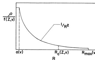
FIG. 2. Model for energy-deposit density as a function of distance from the track of a penetrating ion.
