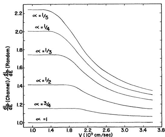
FIG. 6. Calculated values of the ratio of scintillation efficiency (channel-to-random) versus velocity for  $O^{16}$  in NaI(Tl), for a set of values of the stopping-power scaling factor  $\alpha$ .
