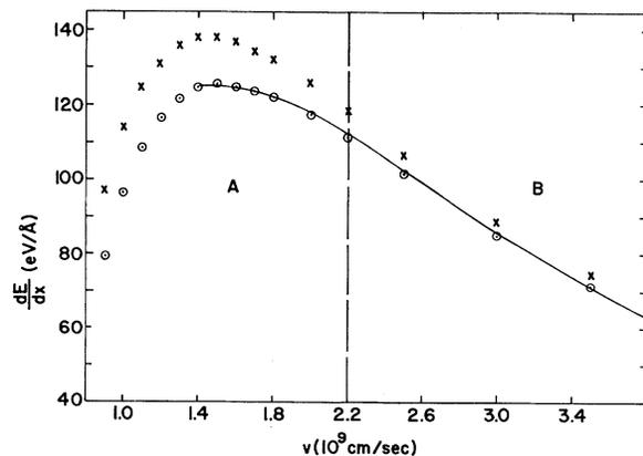
FIG. 3. Specific energy loss versus velocity for  $O^{16}$  ions in NaI: Crosses represent calculated values from Ref. 2, without use of a core correction. Open circles represent values calculated with a core correction. The solid curve represents the semiempirical data of Ref. 3. Regions A and B correspond to intermediate and high velocities, respectively.
