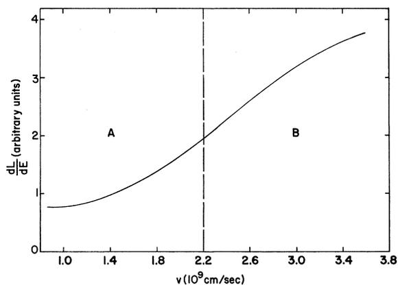
FIG. 1. Data for scintillation efficiency versus velocity for randomly incident  $O^{16}$  ions in NaI(Tl) at room temperature (Refs. 3 and 5). Regions A and B correspond to intermediate and high velocities, respectively.
