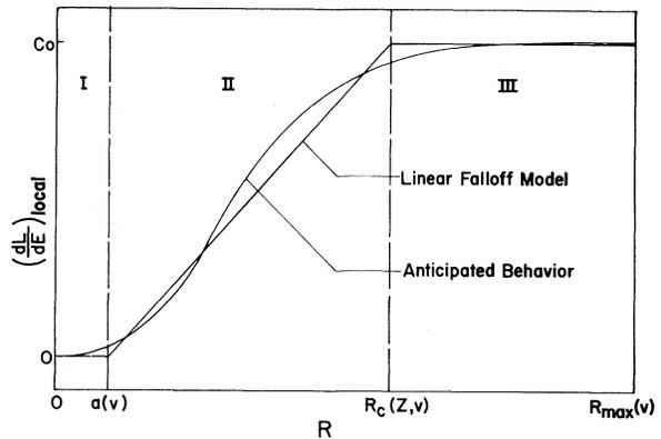
FIG. 4. Model for the local light-production efficiency as a function of distance from the track, superimposed on a curve representing its anticipated behavior. Regions I, II, and III correspond to the immediate vicinity of the track, and the high- and low-density domains, respectively.
