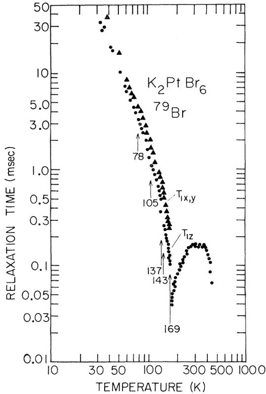
FIG. 3. Temperature dependence of the  $^{79}\text{Br}$  spin-lattice relaxation time in  $\text{K}_2\text{PtBr}_6$ . Only the phase transition at 169 K is clearly apparent in the data.
