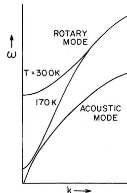
FIG. 5. Theoretical model for the dispersion curve of the rotary lattice mode at 300 and 170 K. The dispersion curve for the acoustic mode is also shown.
