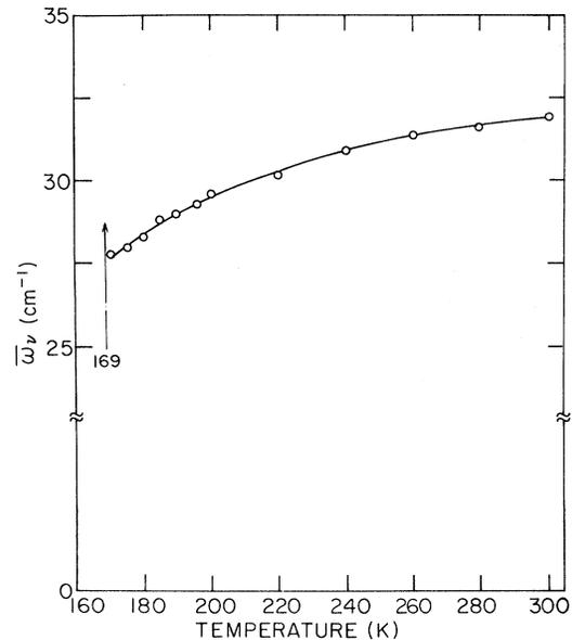
FIG. 2. Temperature dependence of the average rotary-mode frequency  $\bar{\omega}_\nu$  as deduced from the NQR-frequency data in the high-temperature cubic phase. A 12% softening between 300 and 169 K is indicated.
