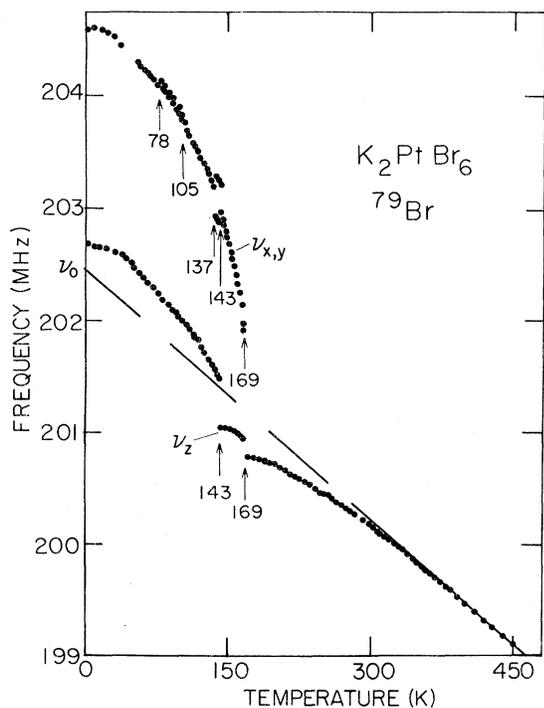
FIG. 1. Temperature dependence of the  $^{79}\text{Br}$  NQR frequency in  $\text{K}_2\text{PtBr}_6$ . The data indicate that five phase transitions occur.
