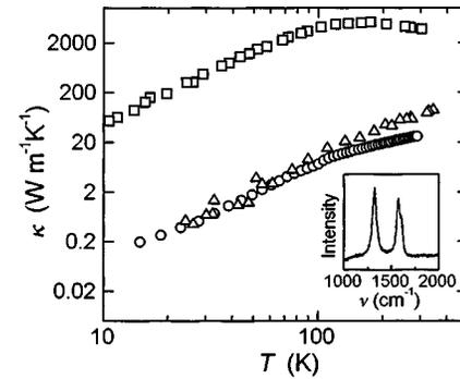
FIG. 3. A log-log plot of the thermal conductivity of our samples (O) compared with that of vapor-grown carbon fibers (Ref. 25) ( $\Delta$ : as-grown,  $\square$ : heat treated at 3000 °C). Inset: First-order Raman spectrum of our MWNT's.
