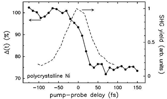
FIG. 4. Ultrafast magnetization breakdown at the surface of bulk Ni in air (solid curve) measured with 65 fs pulses at room temperature. The dashed curve represents the cross-correlation between pump and probe pulses indicating that the breakdown is limited by the pulse width.
