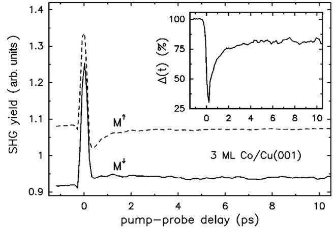
FIG. 2. Total  $p$ - $P$  SHG yield for opposite magnetization directions in transversal geometry as a function of delay between pump and probe pulses for a 3 ML Co film on Cu(001) at 323 K. The inset shows breakdown and recovery of magnetization for an applied  $p$ -polarized pump fluence of  $12 \text{ mJ/cm}^2$ .
