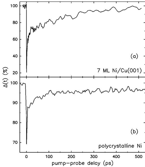
FIG. 3. Recovery of magnetization on a long time scale for (a) 7 ML Ni film on Cu(001) in UHV at 323 K ( $s$ -polarized pump at about  $12 \text{ mJ/cm}^2$ ) and (b) bulk Ni surface in air at room temperature ( $p$ -polarized pump at about  $6 \text{ mJ/cm}^2$ ).
