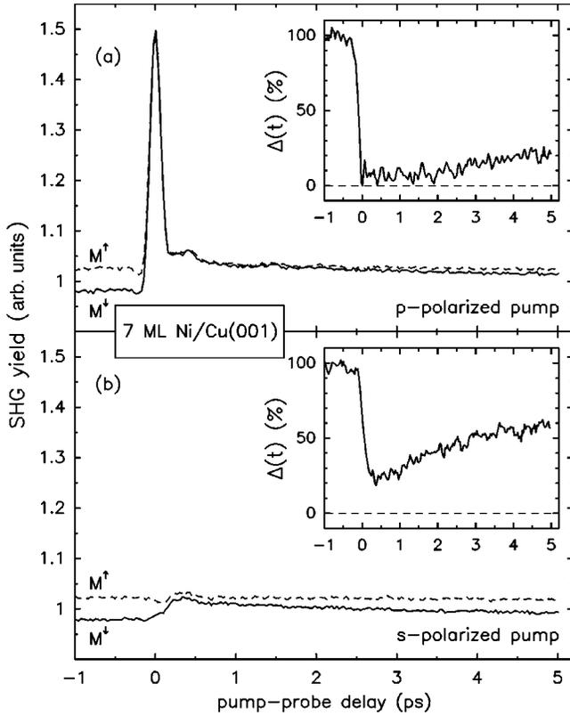
FIG. 1. Total  $p$ - $P$  SHG yield ( $p$ -polarized fundamental and SHG) for opposite magnetization directions in transversal geometry as a function of delay between pump and probe pulses for a 7 ML Ni film on Cu(001) at 323 K. (a) and (b) show the results for  $p$ - and  $s$ -polarized pump light, respectively. The insets show breakdown and recovery of magnetization with the relative difference  $\Delta(t)$  defined in the text. The applied pump fluence was  $12 \text{ mJ/cm}^2$ .
