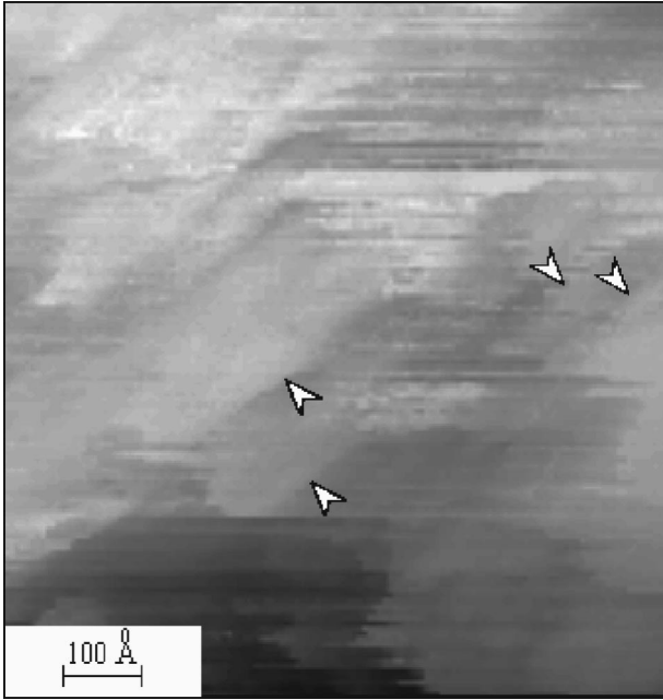
FIG. 4. An 853 \text{ \AA} \times 906 \text{ \AA} image of the LCMO thin film. The image was taken in the constant current mode, with a tip bias of +1.5 \text{ V} and a tunneling current of 2 \text{ nA} . The temperature of the sample was 298 \text{ K} . The atomically smooth terraces are terminated by atomic steps, some of which are marked by the arrows.
