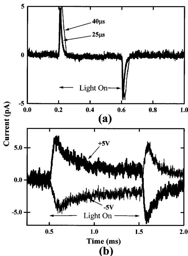
FIG. 3. (a) Transient current responses at zero bias for a 30-nm-thick HMWHC film obtained with different amplifier rise-time values, 40  $\mu$ s (light line) and 25  $\mu$ s (heavy line). (b) Thermal expansion responses at finite biases, +5 V (heavy line) and -5 V (light line).
