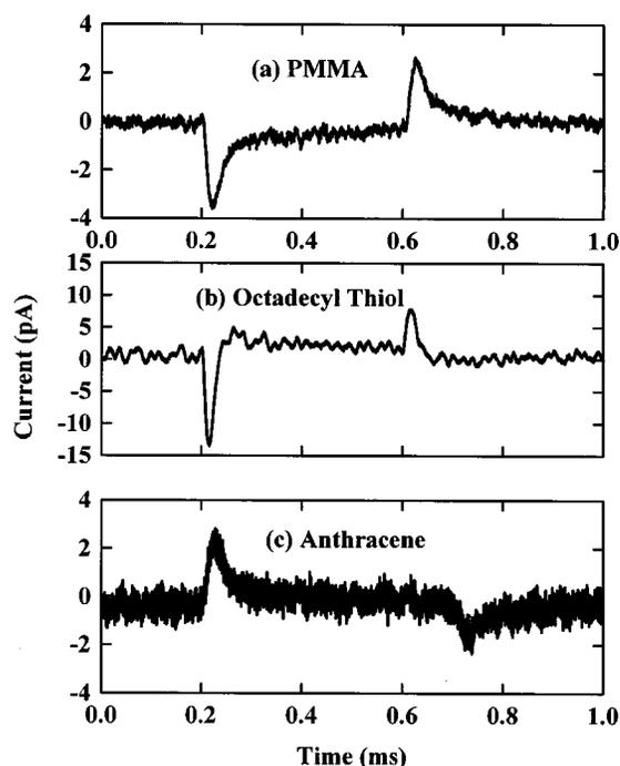
FIG. 7. Transient current responses at zero bias for various sample films: (a) PMMA film approximately 100 nm thick. (b) Octadecanethiol film 2.5 nm thick. (c) Anthracene film about 50 nm thick.
