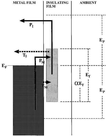
FIG. 5. Energy diagram for the midgap region of the interface between the metal film and the insulating film. Arrows indicate the four current components, which are labeled by the rate constants introduced in the text.
