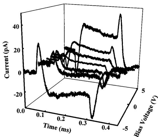
FIG. 6. Bias dependence of the current transients for an approximately 20-nm-thick HMWHC film.
