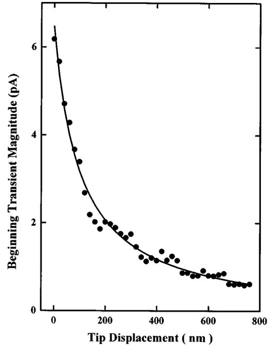
FIG. 4. Dependence of (beginning) transient magnitude on tip position. The zero value for tip position corresponds to the tip being about 20 nm away from the free surface of the insulating film. Fitting the data using the expected inverse relationship of transient magnitude to total tip-sample distance  $d + d_0$  gives the solid line with  $d_0 = 98$  nm. Note weak oscillations of period  $\lambda/2$  due to weak Fabry-Perot behavior of the junction.
