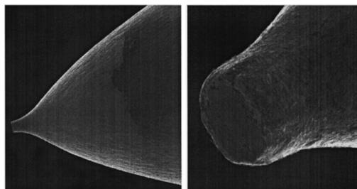
FIG. 2. Scanning electron microscope image of the side and end of a platinum tip with 10- $\mu$ m-diam flat.
