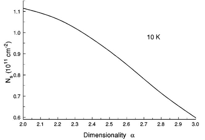
FIG. 2. Total saturation density,  $N_s^\alpha$  as a function of  $\alpha$  in ZnSe/Cd<sub>x</sub>Zn<sub>1-x</sub>Se quantum wells at 10 K.
