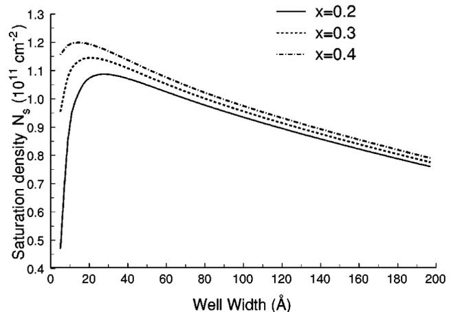
FIG. 1. Total saturation density  $N_s^\alpha$  [Eq. (15)] as a function of the well width in GaAs/Al<sub>x</sub>Ga<sub>1-x</sub>As quantum wells.
