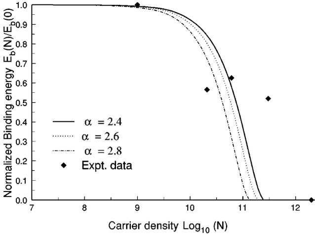
FIG. 4. Diamond-shaped points denote experimental data (Ref. 25) of the normalized binding energy  $[E_b(N)/E_b(0)]$  [Eq. (20)] as a function of sheet carrier density,  $N(\text{cm}^{-2})$  in ZnSe/Cd<sub>0.1</sub>Zn<sub>0.9</sub>Se quantum wells of width 30 Å at 10 K. Solid ( $\alpha=2.4$ ), dotted ( $\alpha=2.6$ ), and dashed-dotted ( $\alpha=2.8$ ) lines are obtained using Eq. (20).
