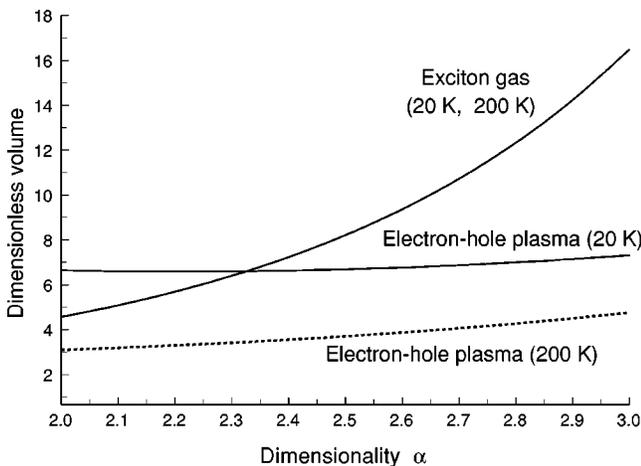
FIG. 5. Dimensionless volume,  $\Lambda_\alpha/[V_\alpha(a_B)]$  [Eqs. (12) and (13)] as a function of dimensionality,  $\alpha$  at 20 and 200 K in GaAs/Al<sub>0.3</sub>Ga<sub>0.7</sub>As quantum wells.
