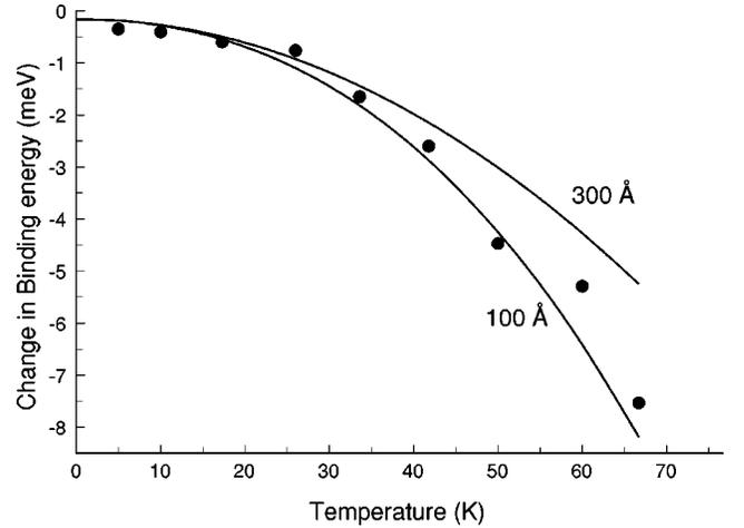
FIG. 6. Dots denote experimental values (Ref. 18) of the change in exciton binding energies with temperature in an  $n$ -type modulation-doped GaAs/Al<sub>0.3</sub>Ga<sub>0.7</sub>As quantum well of width, 100 Å and an electron density of  $1.5 \times 10^{11} \text{ cm}^{-2}$ . Lines at well widths 100 and 300 Å are obtained using Eqs. (12), (13), (15), and (20).
