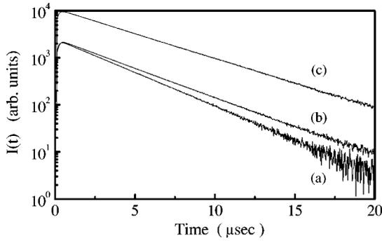
FIG. 1. The real-time signal intensity  $I(t)$  caused by the relaxational mode with  $|\mathbf{q}|=7.5 \times 10^3 \text{ cm}^{-1}$  at  $T=44.6^\circ\text{C}$ . (a)  $\mathbf{q}||a^*$ , (b)  $\mathbf{q}||b$ , and (c)  $\mathbf{q}||c$  axes.
