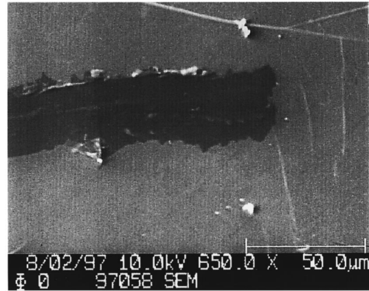
FIG. 6. SEM image of a distinct surface area of a 50-nm-thick Si/Cs/O film having an average cluster size of 5 nm on a HOPG substrate. Here, a small strip of the film has flaked off.
