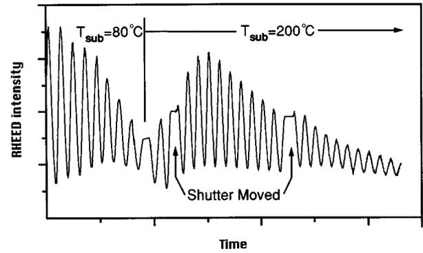
FIG. 3. The RHEED intensity oscillations (second anti-Brag reflection) for Fe growth on a Cr template. This growth was carried out for an Fe-whisker/Cr/Fe(001) sample having three different thicknesses for the deposited Fe layer. The growth was stopped, the shutter was moved, and the growth was again resumed as indicated in the figure.
