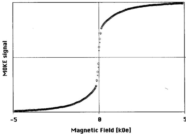
FIG. 9. Longitudinal MOKE signal for the sample Fe/11Cr/3Mn/20Fe/20Au(001).  $J_2 \sim 0.8$  erg/cm<sup>2</sup>,  $J_1 < J_2$ . The rapid change in the MOKE signal around  $H=0$  corresponds to the remagnetization process of the Fe whisker. Note that there is no field region where the magnetic moment of the 20-ML-thick Fe film lies antiparallel to the Fe-whisker magnetization. The ground state is noncollinear.
