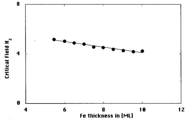
FIG. 10. The critical field  $H_2$  obtained from MOKE measurements as a function of the Fe(001) thickness for an Fe-whisker/11Cr/wedged Fe/20Au specimen. The Cr layer was deposited using optimal conditions for a smooth growth. The wedge-shaped iron film was grown by means of a slowly moving shutter.
