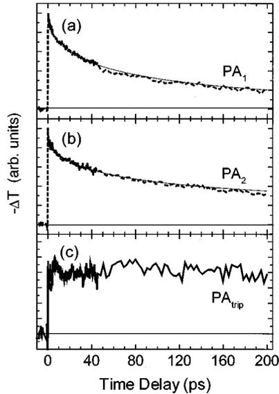
FIG. 2. (a) Normalized time traces of the  $PA_1$  absorption band at 1.59 eV for a pump-pulse energy of 42 nJ. (b) Normalized time traces of  $PA_2$  at a probe energy of 1.8 eV for a pump-pulse energy of 42 nJ (dashed lines). Solid lines are fitted. (c)  $PA_{trip}$  due to actual triplet population (see text).
