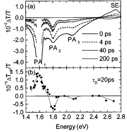
FIG. 1. (a) Conventional transient pump/probe spectra of the polycrystalline PHP film for different pump-probe delays, measured in an OLED structure. (b) The field-induced  $(\Delta T/T)_{\text{MF}}$  spectrum of PHP films for pump-probe delay of  $20 \text{ ps}$  and an applied reverse bias of  $16 \text{ V}$ . Data points are obtained using a monochromator or interference filters. The solid line is a guide to the eye.
