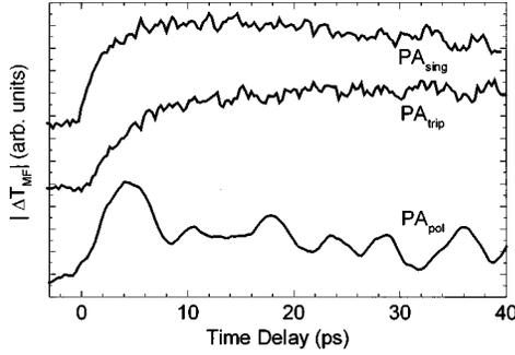
FIG. 4. Normalized field-induced quenching of the singlet absorption ( $PA_{\text{sing}}$ ) at 1.59 eV, increase of the triplet absorption ( $PA_{\text{trip}}$ ) at 1.8 eV, and increase of the polaron absorption ( $PA_{\text{pol}}$ ) at 2.09 eV for an applied reverse bias of 16 V and a pump-pulse energy of 160 nJ. Traces are vertically displaced for clarity.
