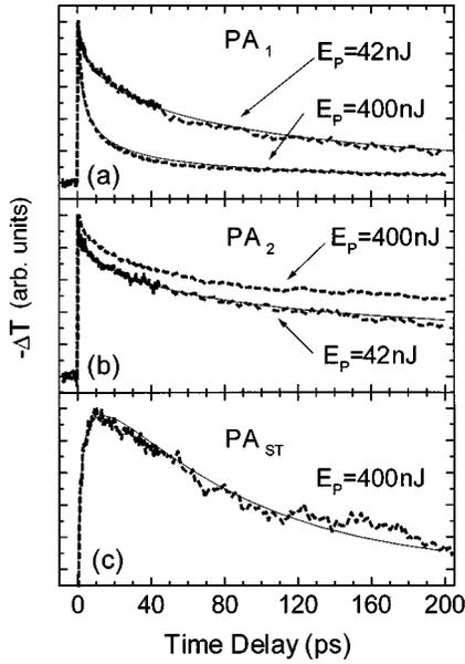
FIG. 6. (a) Normalized time traces of the  $PA_1$  absorption band at 1.59 eV for different pump-pulse energies (dashed lines). (b) Normalized time traces of  $PA_2$  at a probe energy of 1.8 eV for different pump-pulse energies (dashed lines). (c) PA due to the additional short-living triplet population  $\Delta n_T$  ( $PA_{ST}$ ) (see text). The smooth curves are calculated according to the rate equations in the text.
