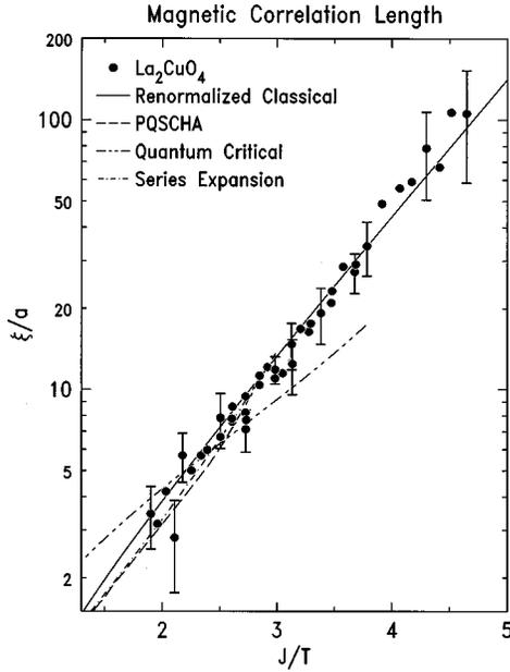
FIG. 8. The logarithm of the reduced magnetic correlation length  $\xi/a$  versus  $J/T$  compared with the predictions of various theories including renormalized classical behavior, Eq. (6), quantum critical behavior, Eq. (11), the PQSCHA, Eq. (10), and high-temperature series expansion (Ref. 29).
