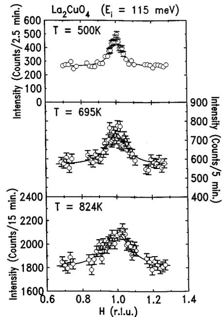
FIG. 4. Representative energy-integrating two-axis scans in  $\text{La}_2\text{CuO}_4$  with  $E_i = 115$  meV and collimations  $20' - 10' - S - 10'$ . The solid lines are the results of fits to a 2D Lorentzian scattering function convoluted with the resolution function of the spectrometer.
