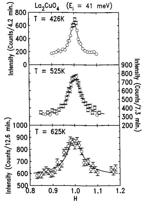
FIG. 3. Representative energy-integrating two-axis scans in  $\text{La}_2\text{CuO}_4$  with  $E_i = 41$  meV and collimations  $20' - 10' - S - 10'$ . The solid lines are the result of fits to a 2D Lorentzian scattering function Eq. (5) convoluted with the resolution function of the spectrometer.
